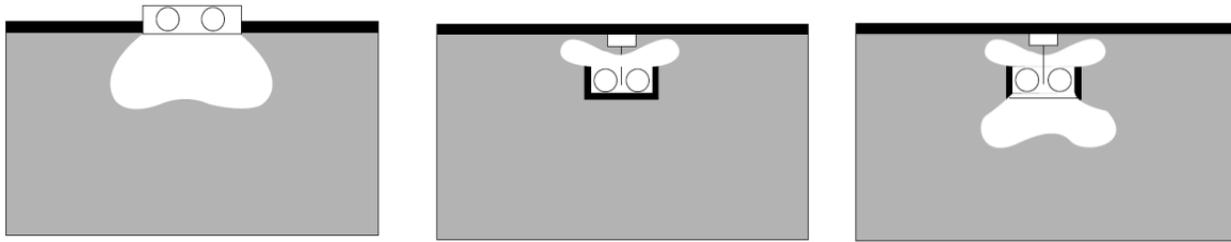
Figure 30: Illustrations of typical candlepower distribution for different ceiling-mounted lighting designs; left, direct lighting; center, indirect lighting; right, direct/indirect lighting
