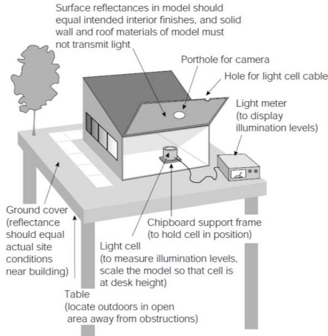
Figure 17: Scale models studied outdoors show the quality of lighting, flag glare problems, and provide measured daylight readings. Source: *Concepts in Architectural Lighting*, by M. D. Egan, McGraw-Hill, 2001.
