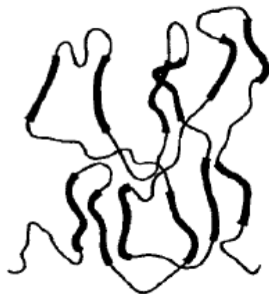
Fig. 5.7 The 'solidification model' of the crystallisation process, showing how a chain can be incorporated into a lamellar structure without significant change of overall shape. (Reproduced by permission of IUPAC.)
