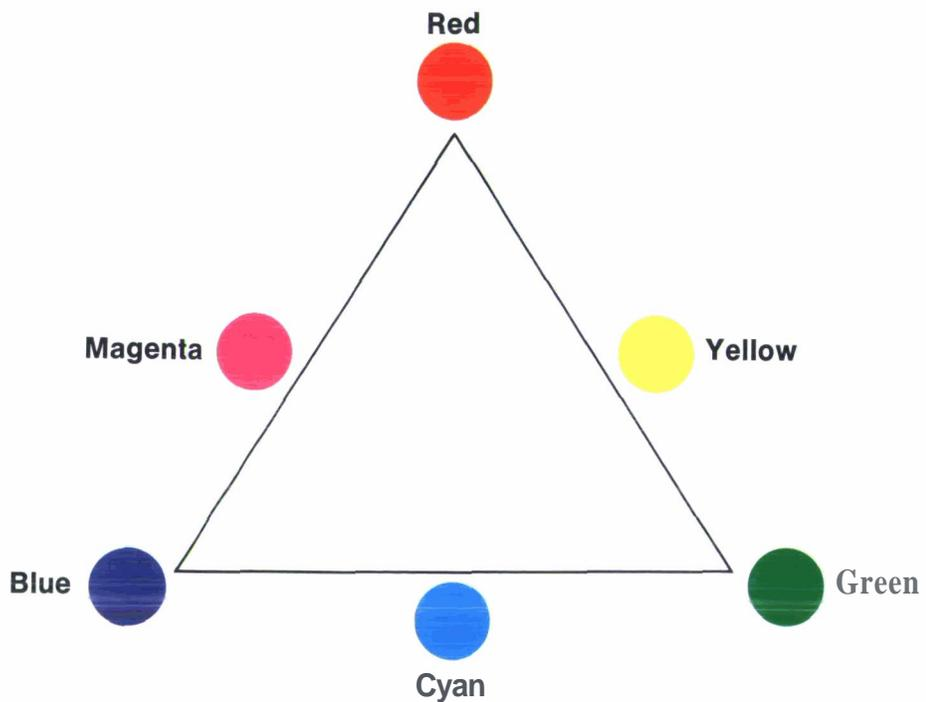
The **additive primary colors** of red, green, and blue are on the points of the triangle. The subtractive primary colors of **cyan, magenta,** and **yellow** are on the sides of the triangle. On this triangle, any two adjacent colors form the one in the middle.
