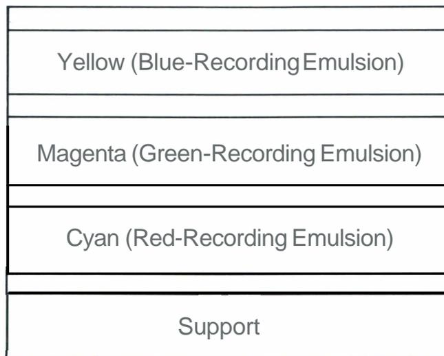
Color films generally have the red-recording layer at the bottom, the **green**-recording layer next, and the blue-recording layer on top. All silver halide crystals are sensitive to blue light. To keep blue light from being recorded in emulsion layers where it isn't wanted, a yellow filter layer is added to the film.
