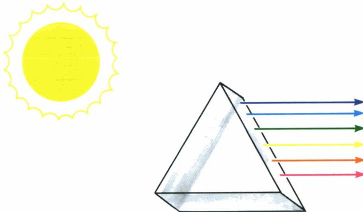
The prism bends the rays of white light at different angles, so the white light is separated into rays of different wavelengths. Each wavelength gives your eye a sensation of different color—a color pattern like a rainbow.
