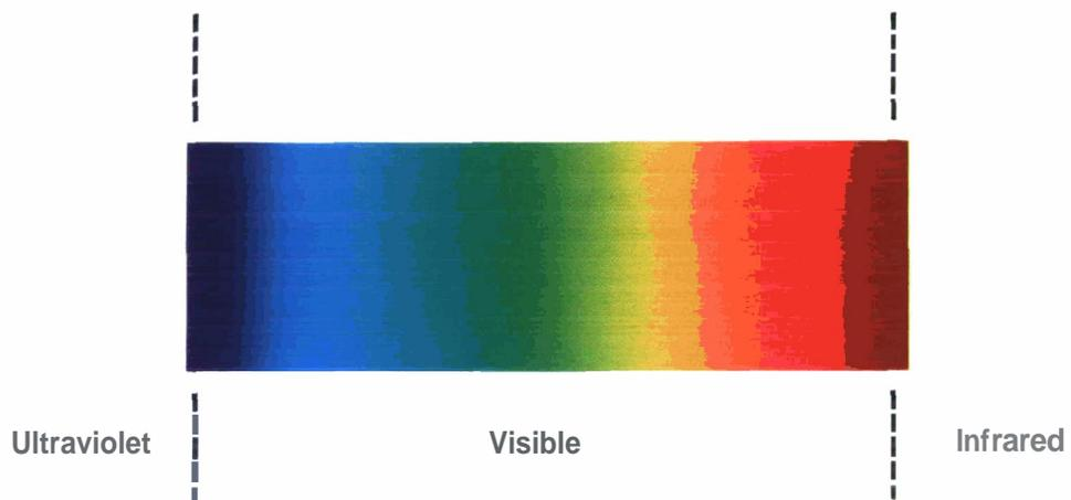
The electromagnetic spectrum is made up of both visible and invisible rays. Only the visible rays in the middle of the spectrum are called light.
