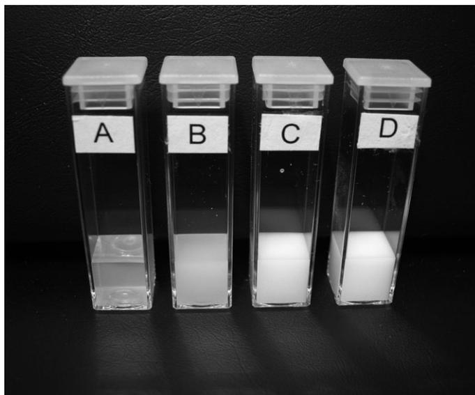
Figure 4. Photograph of cuvettes containing various volume fractions (A =  $2.36 \times 10^{-5}$ , B =  $2.36 \times 10^{-4}$ , C =  $4.728 \times 10^{-4}$  and D =  $7.092 \times 10^{-4}$ ) of the  $\text{TiO}_2$  dispersed in 10 mM NaCl.
