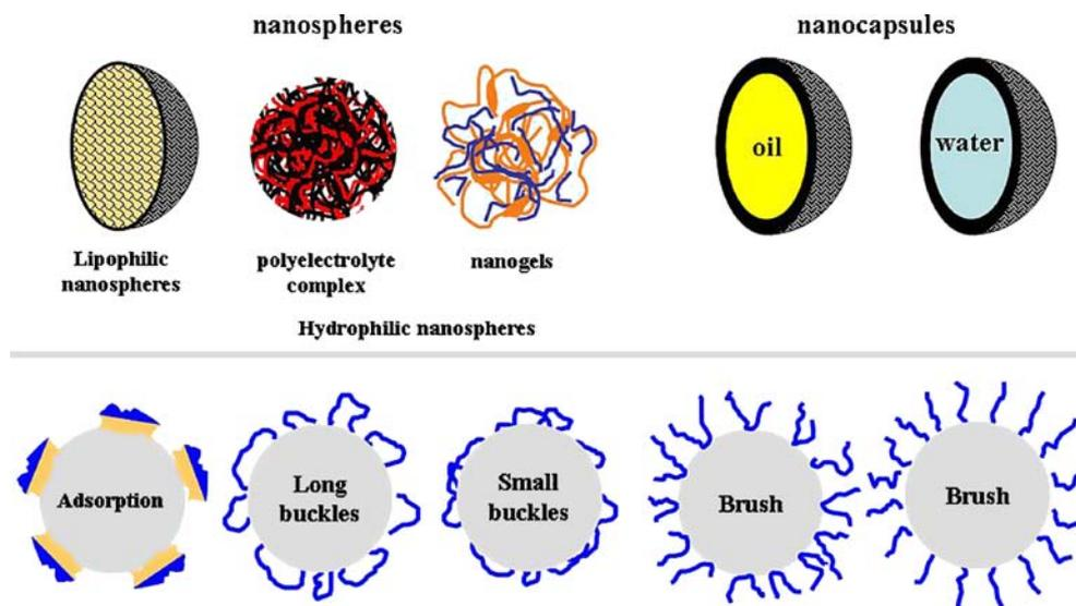
**Fig. 1.** Structure of the different types of polymer nanoparticles (*upper part*) and steric arrangement of coating material made of amphiphilic block copolymers of different structures (*lower part*).
