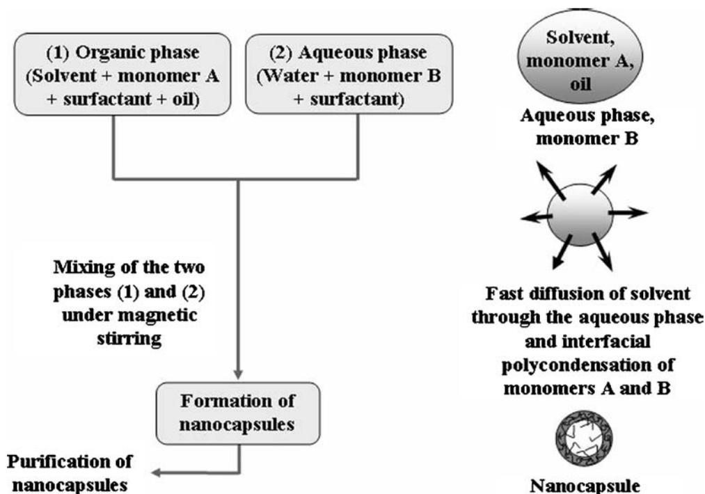
**Fig. 8.** Preparation of nanocapsules by interfacial polycondensation combined with spontaneous emulsification and hypothesis about the mechanism of formation. [adapted from (25)]. (1) Organic phase: organic solvent (40 mL), lipophilic monomer (A), oil (400 mg), lipophilic surfactant (86 mg of Span<sup>®</sup>85). (2) Aqueous phase: water (80 mL), hydrophilic monomer (B), hydrophilic surfactant (136 mg of Tween<sup>®</sup>20).
