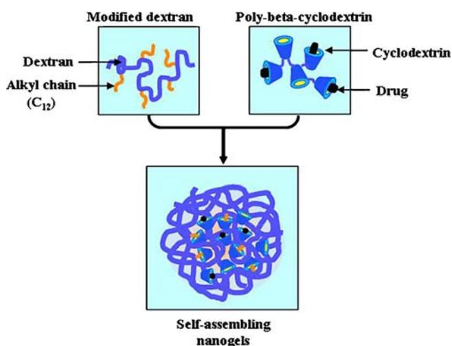
**Fig. 9.** Schematic representation of formation of nanogels by self-assembly of neutral macromolecules. The concentration of the polymer in the suspension of nanogels ranges from 2.5% to 7.5% (w/w) and the ratio of the two polymers modified dextran/poly-beta-cyclodextrin varied from 20/80 to 80/20 (w/w) [adapted from (164)].
