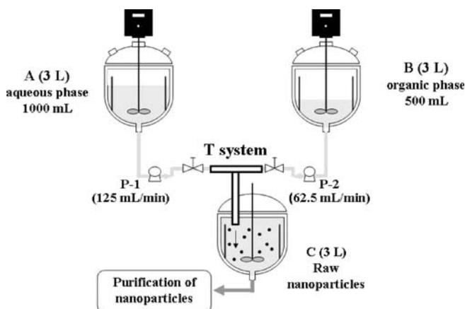
**Fig. 14.** Pilot set up proposed for the scaling-up of nanoparticle production by the nanoprecipitation method. P-1 and P-2 are peristaltic pumps working at flow rates indicated in the parenthesis [adapted from (202,204)].
