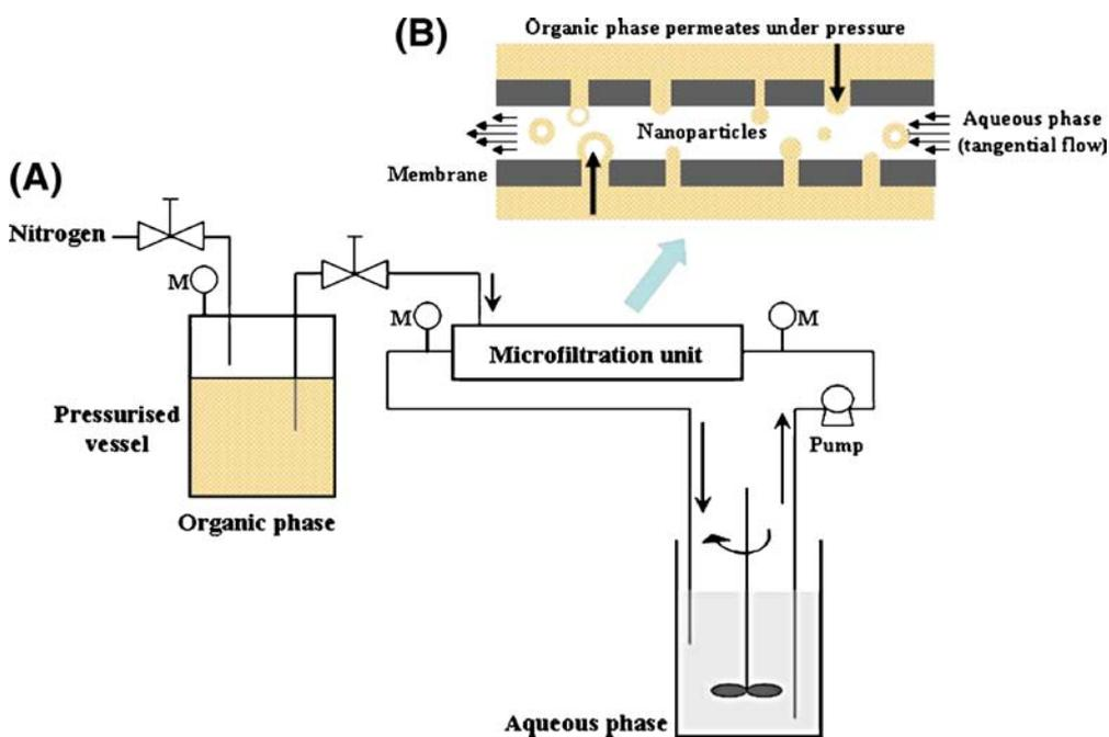
Fig. 3. Experimental set-up for the nanoparticle preparation using membrane contactor. **A** General set up. *M* Manometer. **B** Enlargement of the microfiltration unit. The aqueous phase which circulates in the microfiltration unit sweeps away droplets of organic phase which form at the pore outlet.
