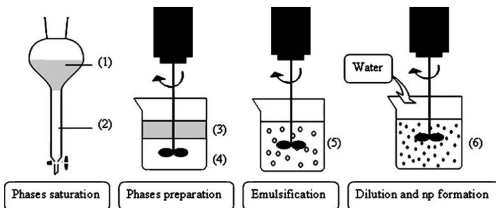
**Fig. 6.** Sketch of the manufacturing of nanoparticles (*np*) by the emulsification–solvent diffusion method. (1) Partially water miscible solvent saturated with water. (2) Water saturated with solvent. (3) Organic phase composed of polymer (2% *w/w*) and oil (5% *w/w*) in (10 mL) of phase (1). (4) Aqueous phase composed of water (40 mL) and surfactant (2.5% *w/w*). (5) Emulsification. (6) Dilution with 200 mL of water.
