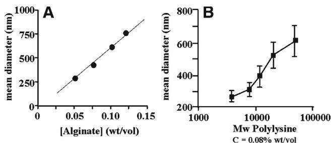
Fig. 10. Effect of the concentration in alginate (A) and of the molecular weight of polylysine (B) on the diameter of the alginate nanoparticles obtained by ionic gelation (168).
