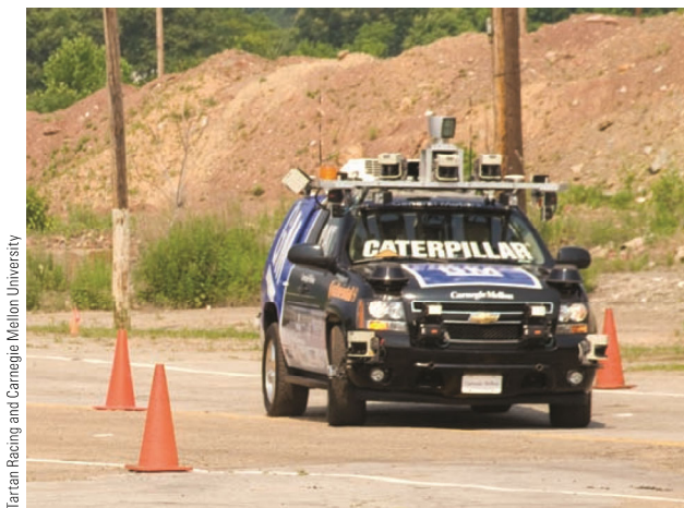
Figure 5.2 ■ The “Boss” robotic vehicle on a test run on a track at Robot City in Pittsburgh. Notice that there is no human driver. Navigation is accomplished by onboard computers that receive information from numerous sensors on the vehicle, each of which has a specialized task. Sensors mounted on the back of the roof are laser range scanners that point down to detect lane markings. Sensors on the roof rack point down crossroads to detect and track vehicles when attempting to merge with traffic. The black sensors on the hood at the front of the vehicle are multiplane, long-range laser scanners used for tracking vehicles. The two white sensors on the corners of the front bumper are short-range laser scanners used to detect and track nearby vehicles. The four rectangles in the grill are radar sensors. The white sensors are short-range, used for detecting obstacles near the vehicle. The black sensors are long-range, for tracking vehicles when Boss is moving quickly or considering turning across traffic.
