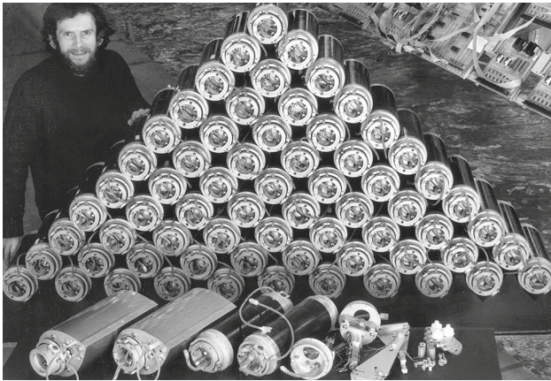
Fig. 9 David Jeffrey with the complete spine model. Beam elasticity could be varied electronically from the control bench. Two illicit generic absorbers can be seen, lower left
