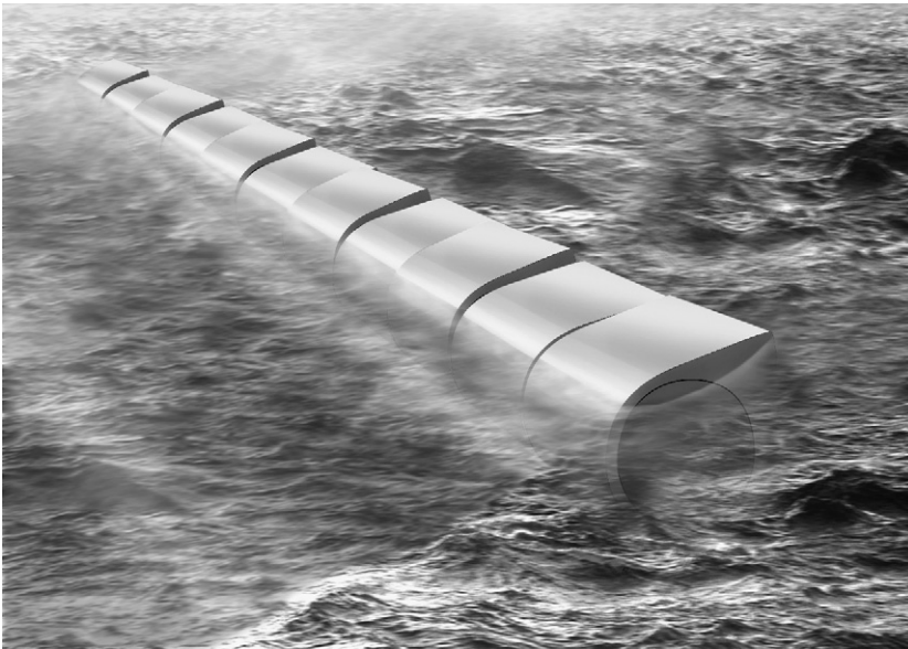
Fig. 4. A set of nodding-duck shaped bodies, performing pitch oscillation, with different phases. Wave-induced pitch moments react against a common cylindrical spine. The relative motion is utilised to run a hydraulic power take-off machinery (not shown).
