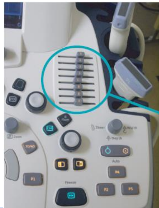
Fig. 4.4 Time-gain compensation (TGC). (a) The gain applied by the TGC amplifier increases with time after transmission to compensate for the greater attenuation of echoes from larger depths. (b) After TGC, echoes from similar interfaces should be equal in amplitude regardless of depth.
