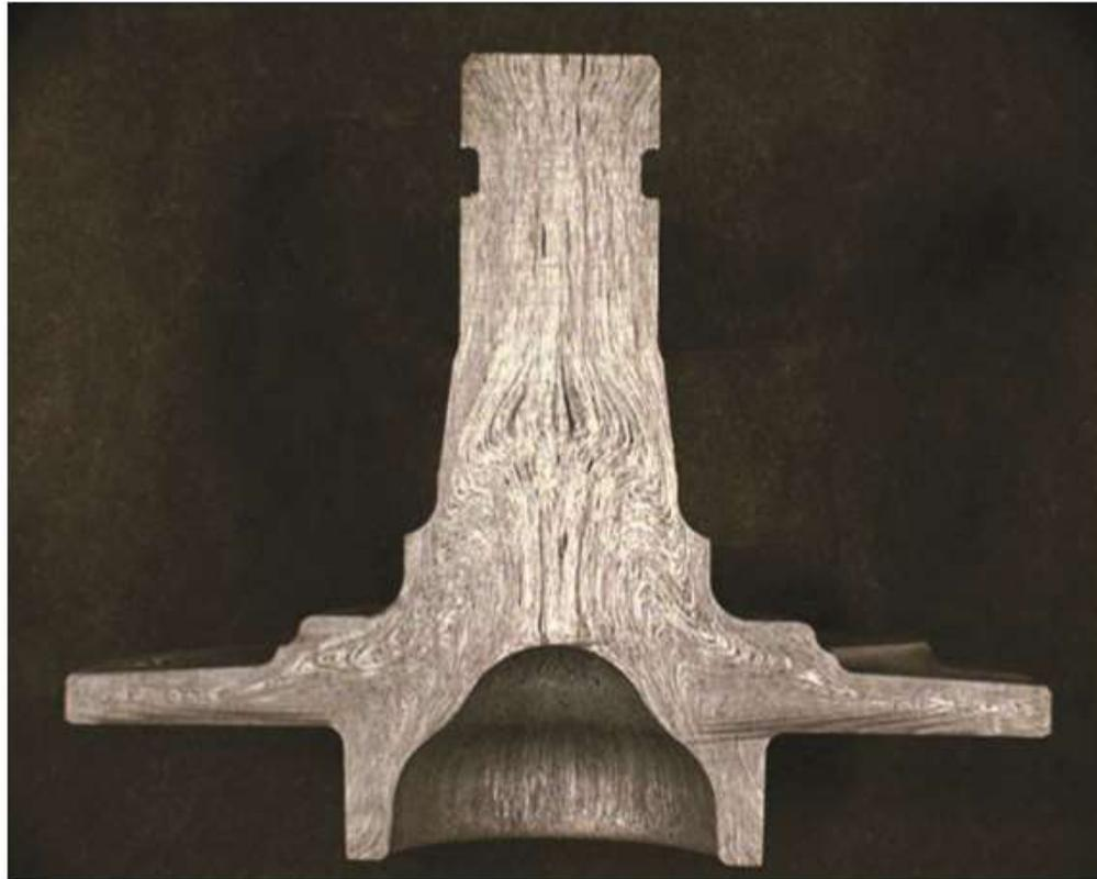
**Figure 1.** Grain flow can be observed in this sliced section of a forging. It has been cut, polished and etched with an acid solution. The observed flow lines are due primarily to the particles and inclusions, which were remnants of the original casting. These have been deformed during the billet conversion and forging process. The forging process has also aligned the grains of the metal in a direction similar to the flow lines in this picture. *(Courtesy HHI Forgings)*
