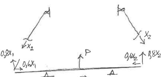
$$\begin{aligned} F_{11} &= \left(\frac{1^2 5a^3}{25EI}\right) + \frac{3a}{3EI} \left(\frac{12}{5}a\right)^2 + \frac{6a}{3(2EI)} \left(\frac{12}{5}a\right)^2 \\ &= \left(\frac{3}{5} + \frac{144}{25} + \frac{144}{25}\right) \frac{a^3}{EI} = \frac{303}{25} \frac{a^3}{EI} \end{aligned}$$
