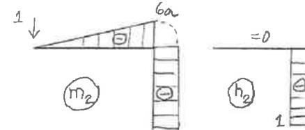
$$u_A = \sum_{b=1}^{m_b} \left[ \frac{\alpha(\Delta T_2 - \Delta T_1)}{h} \int m_1 dx + \alpha \Delta T_2 \int h_1 dx \right] = \frac{\alpha(-\Delta T)}{2} (2a \times 4a) + \alpha \left( \frac{\Delta T}{2} \right) (-1 \times 6a)$$
