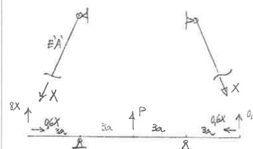
$$\begin{aligned} F_{11} &= \sum_{b=1}^6 \left[ \left( \frac{m_1 n_1}{EA} + \frac{m_1 m_1}{EI} \right) dx \right] \\ &= 2 \times \left( \frac{1^2 a^2}{25EI} \right) + 2 \times \left( \frac{3a}{5} \left( \frac{12}{5} a \right)^2 \right) \\ &+ \frac{6a}{(2EI)} \times \left( \frac{12}{5} a \right)^2 = \frac{750}{25} \frac{a^3}{EI} \\ d01 &= 2 \left( -\frac{3a}{2(2EI)} \left( \frac{12}{5} a \times \frac{3Pa}{2} \right) \right) = -\frac{54}{10} \frac{Pa^3}{EI} \end{aligned}$$
