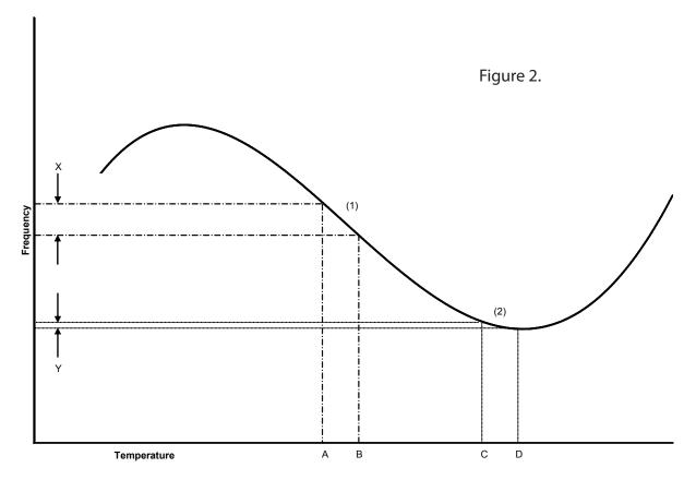
As shown above, the actual temperature to which the oven is set is critical in minimizing the effect of ambient temperature change.
