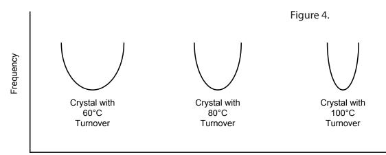
Second, and more important, crystal aging (discussed below) degrades with an increasing temperature. Therefore, in designing an oven controlled crystal oscillator, one is faced with a compromise in determining the desired oven operating temperature; it should be low as practicable, but it must be high enough to provide good control at the maximum ambient operating temperature.
