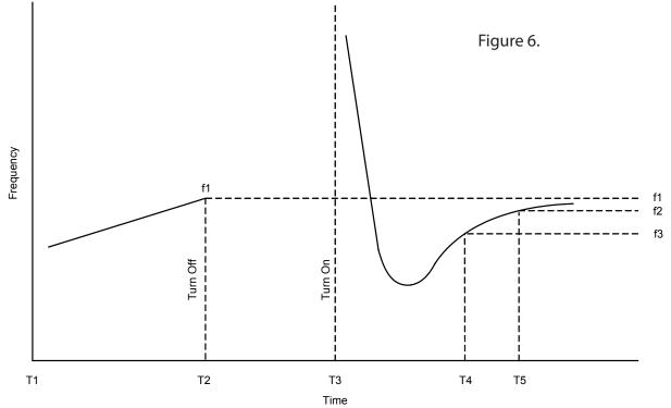
In Figure 6, assume that an oscillator is energized until time T2 when it is turned off for a period of time and then turned on again at time T3. Three characteristics may then be of significance:
