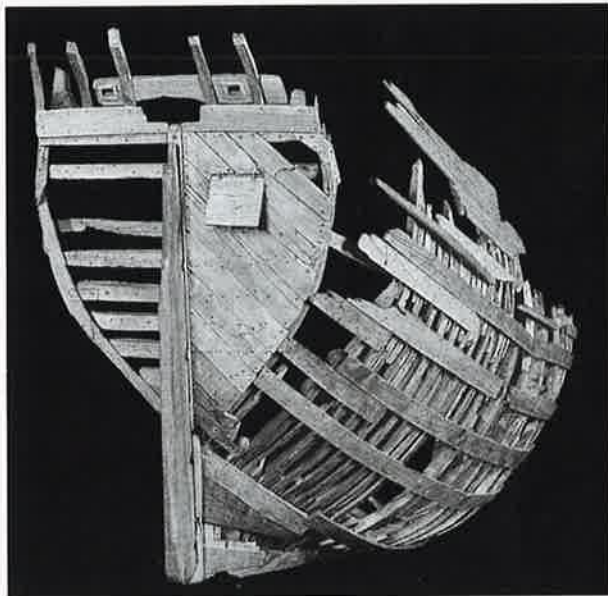
Model, at a scale of 1:10, to show how the galleon's surviving timbers may have fitted together. The outline of the ship now forms part of the logo of the UNESCO 2001 Convention on the Protection of the Underwater Cultural Heritage (below).
