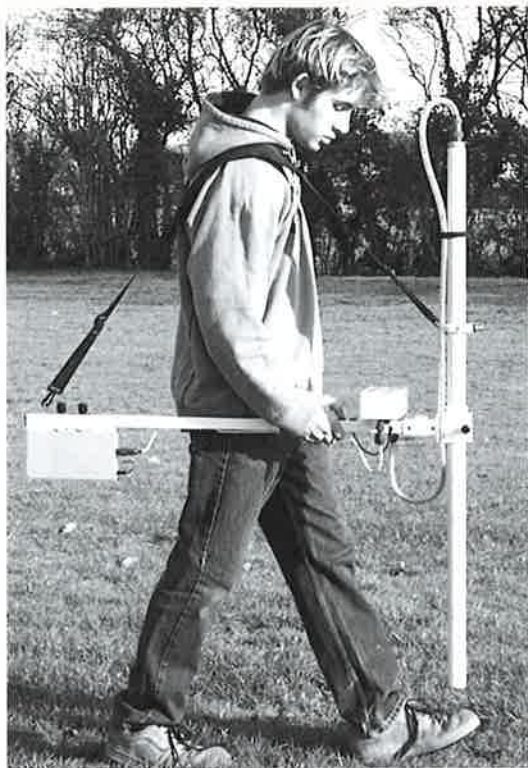
The Bartington Grad 601/1 single vertical component high stability fluxgate gradiometer, capable of 10 readings per second with a resolution of 0.1nT/m.
