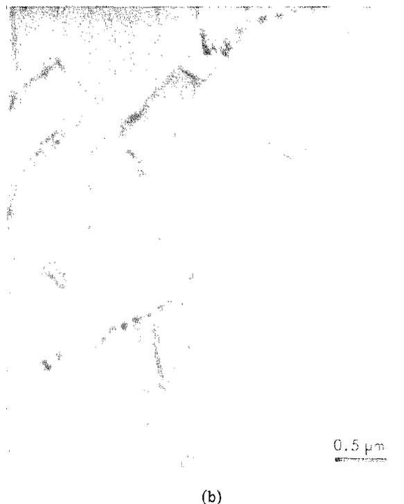
Fig. 18.2 Microstructure of unirradiated type 304 stainless steel (a) Photomicrograph showing grain structure. (b) Electron micrograph showing dislocation structure. (From E. E. Bloom, An Investigation of Fast Neutron Radiation Damage in An Austenitic Stainless Steel, USAEC Report ORNL-4580, Oak Ridge National Laboratory, 1970.)
