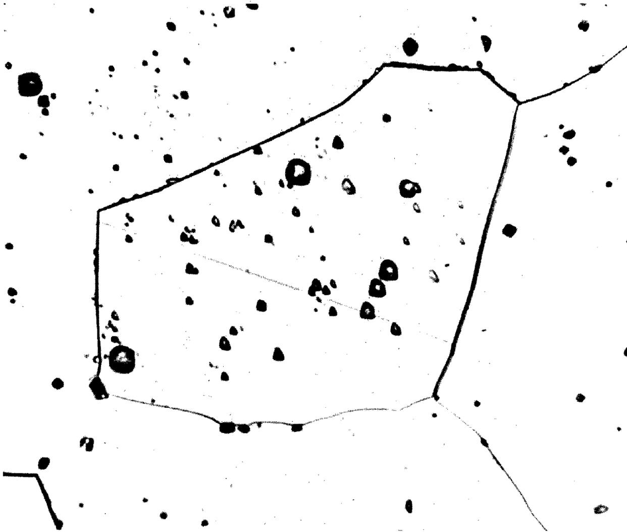
Fig. 14.14 Grain structure in UO<sub>2</sub> in which some grain growth has occurred. The grain in the center is 50  $\mu\text{m}$  in size. [From J. R. MacEwan and J. Hayashi, *Proc. Brit. Ceram. Soc.*, 7: 245 (1967).]
