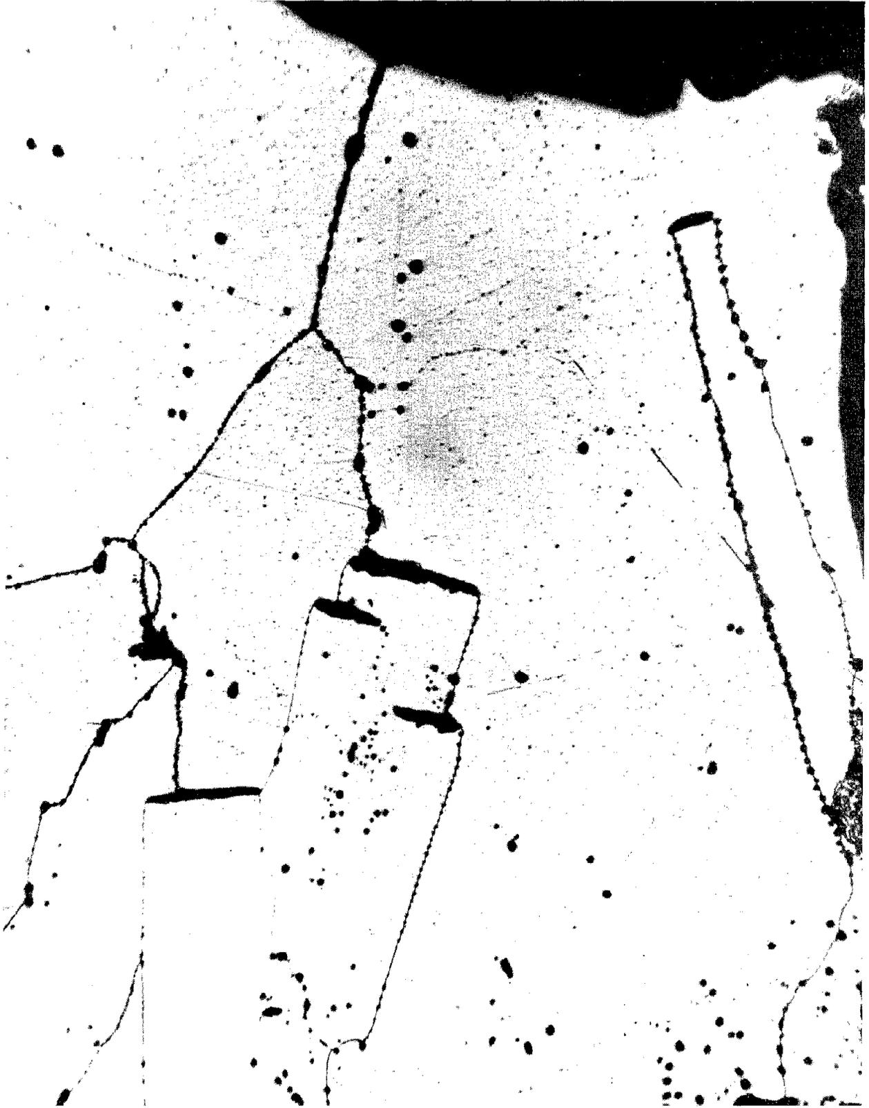
Fig. 14.4 Lenticular pores moving toward the center of the fuel (top right) leaving behind series of small spherical pores or bubbles. [From F. A. Nichols, *J. Nucl. Mater.*, 27: 137 (1968).]
