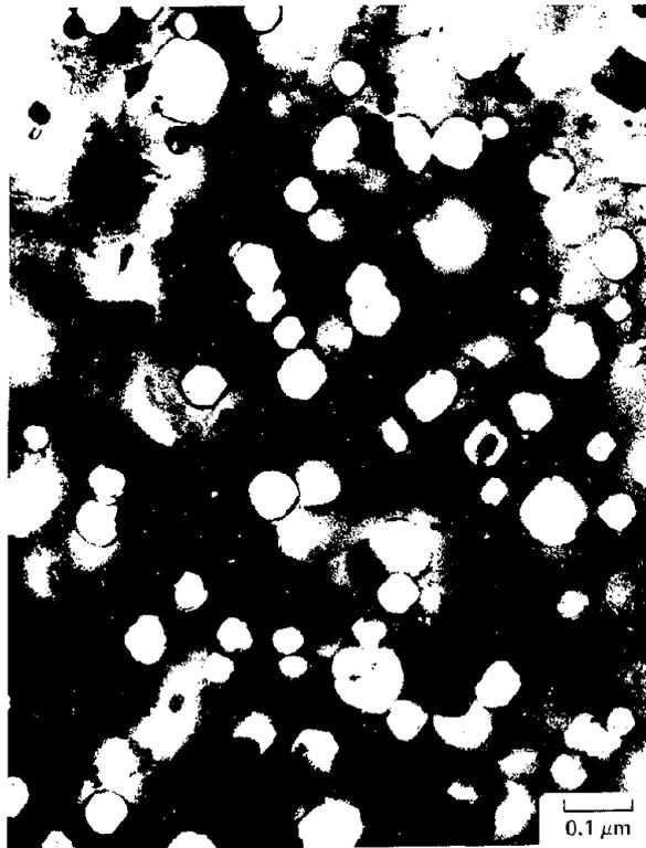
Fig. 18.6 Type 316 stainless-steel specimen irradiated at 525°C to  $7.1 \times 10^{22}$  neutrons/cm<sup>2</sup> ( $E > 0.1$  MeV). Mean void diameter, 640 Å; void number density,  $4.4 \times 10^{14}$  voids/cm<sup>3</sup>. [From W. K. Appleby et al., in *Radiation-Induced Voids in Metals*, Albany, N. Y., James W. Corbett and Louis C. Ianniello (Eds.), USAEC Symposium Series, CONF-710601, p. 166, 1971.]
