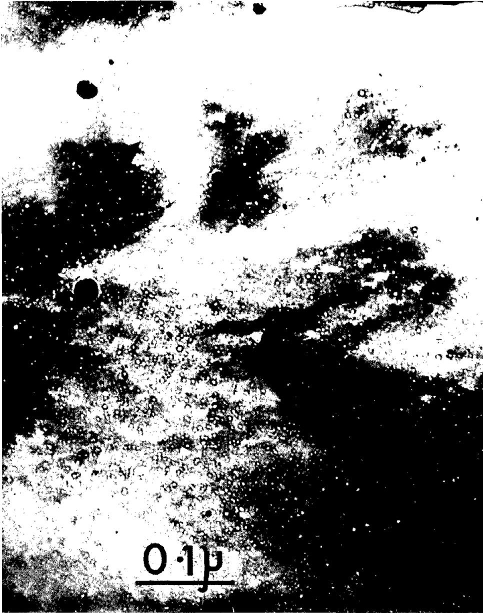
Fig. 13.14 Micrographs showing intragranular fission-gas bubbles. Note how many of them lie in straight lines. [From J. A. Turnbull, *J. Nucl. Mater.*, 38: 206 (1971).]
