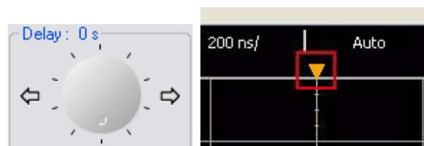
Figure D-15 – Soft Front Panel of the Delay Control and Trigger Point
