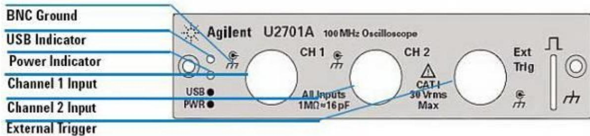
Figure D-6 – Front Panel of the U2701A
