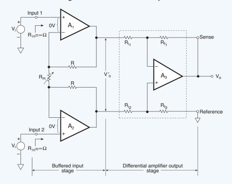
**Fig. 5.11.** The instrumentation amplifier exhibits extremely high impedance to the inputs  $V_1$  and  $V_2$ . Resistor  $R_m$  adjusts the gain, and the single-ended output is a function of the difference between  $V_1$  and  $V_2$ .
