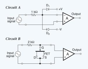
**Fig. 5.35.** Certain CMOS multiplexers may be protected against overvoltage destruction with diode and resistor networks that shut down any parasitic transistors in the device, limit the current input to a safe level, and shunt input signals to ground when the power supplies are turned off (Circuit A). JFET transistors also protect multiplexer inputs when they are connected as diodes. The JFET clamps at about 0.6V, protecting the sensitive op amp input from destruction (Circuit B).
