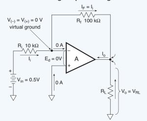
**Fig. 5.05.** The output polarity of the inverting amplifier is opposite to that of the input voltage. The closed-loop amplification or gain of this stage is  $A_{cl} = 10$ , which is the ratio of  $R_f/R_i$  or 100 k $\Omega/10$  k $\Omega$ .
