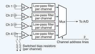
**Fig. 5.13C.** A typical production type data acquisition system contains an instrumentation amplifier and a low-pass filter in each channel preceding the MUX. The amplifier boosts low-level signals sufficiently well to let the active filter work at an optimum signal-to-noise ratio.
