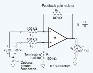
**Fig. 5.07.** The output voltage of the basic differential amplifier is the difference between the two inputs, or  $A_{cl} = g(V_1-V_2)$ , where g is the gain factor. Because all resistors in this example are of equal value, the gain is unity. However, a gain of 10 may be obtained by making the feedback resistor 10 times larger than the input resistors, under the conditions that both feedback resistors are equal and the input resistors are equal.
