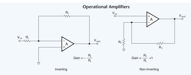
**Fig. 5.04.** *The two basic types of operational amplifiers are called inverting and non-inverting. The stage gain equals the ratio between the feedback and input resistor values.*
