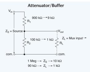
**Fig. 5.17.** When the input signal exceeds about 10V, the divider drops the excess voltage to prevent input amplifier damage or saturation.
