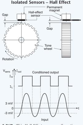
**Fig. 5.26B.** This Hall-Effect sensor configuration uses a bias magnet and a tone wheel that modulates the magnetic field intensity to produce an output signal.
