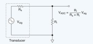
**Fig. 5.03A.** The sensor's source impedance  $R_s$  should be relatively small to increase the voltage divider drop across  $R_i$ , the amplifier's input. This can substantially improve the signal-to-noise ratio for mV range sensor signals.
