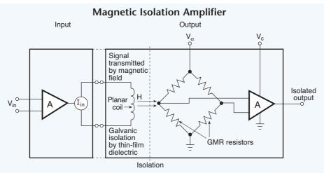
**Fig. 5.24A.** Magnetic couplers transfer signals through a magnetic field across a thin film dielectric. In this case, a magnetoresistance bridge circuit sensitive to the field exhibits a large change in resistance when exposed to the magnetic field from a small coil sitting above it.
