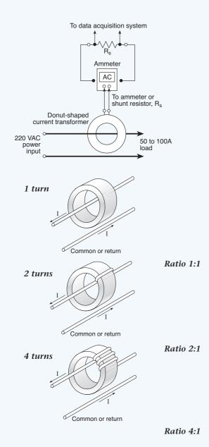
**Fig. 5.27.** Because it does not need a ground connection, a current transformer is isolated from both the input and output of the signal conditioner.
