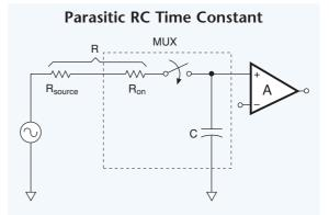
**Fig. 5.02.** The source resistance should be as low as possible to minimize the time constant of the MUX's parasitic capacitance C and series resistance R. An excessively long time constant can adversely affect the circuit's measurement accuracy.
