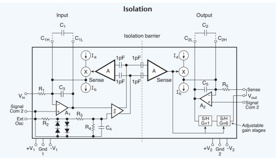
**Fig. 5.20.** A differential isolation amplifier's front end can float as high as the value of the common mode voltage (CMV) rating without damage or diminished accuracy. The isolation barrier in some signal conditioners can withstand from 1,500 to 2,200 VDC.
