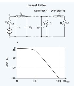
Fig. 5.12C. Bessel filter and response characteristics
