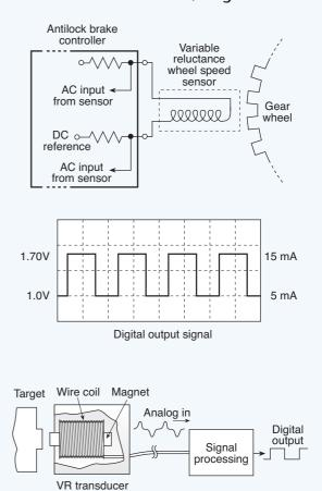
**Fig. 5.28.** Variable reluctance sensors comprise a coil of wire wound around a magnetic core. As a ferrous metal passes near one pole it disturbs the magnetic field and induces a small voltage in the coil. In this example, the voltage is amplified, shaped, and converted to a digital signal for indicating vehicle wheel speed.
