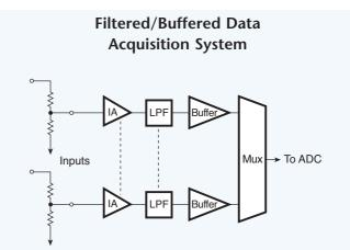
**Fig.5.13A.** An instrumentation amplifier, a low-pass filter, and a unity gain buffer amplifier placed between the sensor output and MUX input transforms the sensor's high output impedance to a low impedance. This is required by the MUX to maintain accuracy.
