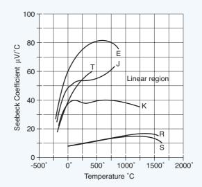
**Fig. 5.30.** The slope of the Seebeck coefficient plotted against temperature clearly illustrates that the thermocouple is a non-linear device.
