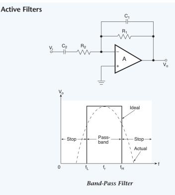
**Fig. 5.15.** *Passive filters tend to change in frequency-cutoff characteristics with a change in load. To prevent this, an active device such as a transistor or op amp isolates the last pole from the load to maintain stable filter characteristics.*
