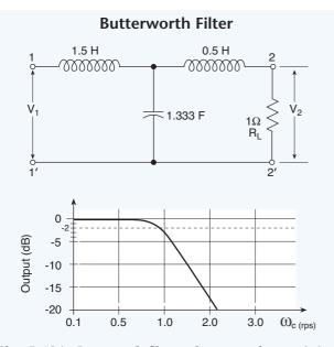
Fig. 5.12A. Butterworth filter and response characteristics
