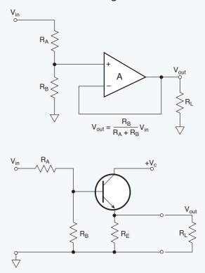
**Fig. 5.18.** *An op amp or a transistor serves as an impedance matching buffer to prevent the load from affecting the divider's output voltage.*
