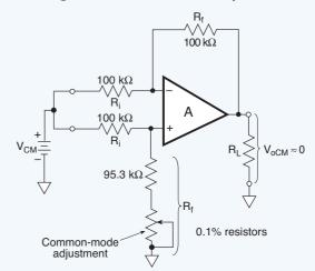
**Fig. 5.10.** The common mode voltage rejection is measured with the two inputs shorted together and a voltage applied to the node. The potentiometer is then adjusted for minimum ( $V_{OCM}$ ) output from the amplifier, signifying that the best balance was reached between the two inputs.
