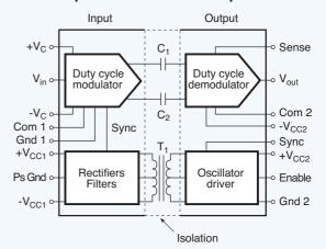
**Fig. 5.22.** The isolation barrier in this amplifier protects both the signal path and the power supply from CMV breakdown. The signal couples through a capacitor and the power through an isolation transformer.
