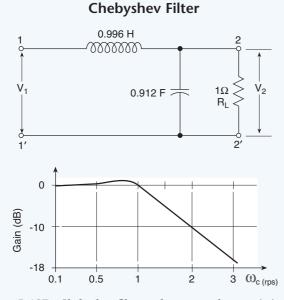
Fig. 5.12B. Chebyshev filter and response characteristics
