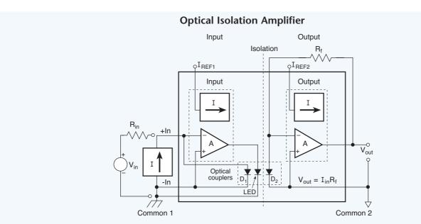
**Fig. 5.23.** This is a simplified diagram of a unity gain current amplifier using optical couplers between input and output stages to achieve isolation. The output current passing through the feedback resistor ( $R_f$ ) generates the output voltage.
