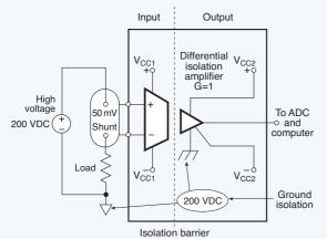
**Fig. 5.21.** *Galvanic isolation can use any one of several techniques to isolate the input from the output circuitry. The goal is to allow the device to withstand a large common mode voltage (CMV) between the input and output signal and power grounds.*
