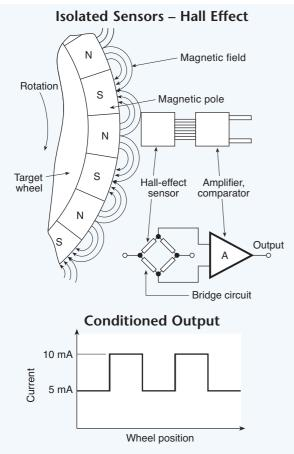
**Fig. 5.26A.** This Hall-Effect sensor is switched with a series of alternating magnets in a target wheel. Each pass between N and S magnets changes the sensor's state.
