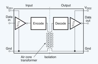
**Fig. 5.25.** Yet another isolation method specifically intended for digital circuits employs a high-speed CMOS encoder and decoder at the input and output, coupled with a monolithic air-core transformer.
