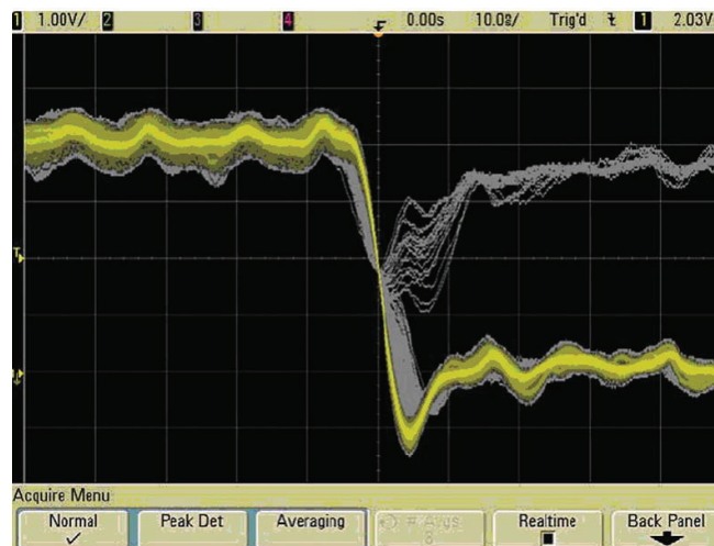
Figure 19. An infrequent glitch caught on an Agilent InfiniiVision 6000 Series oscilloscope
