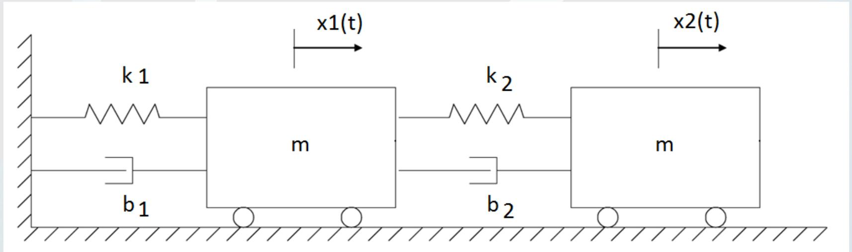
$$\underbrace{\begin{bmatrix} m_1 & 0 \\ 0 & m_2 \end{bmatrix}}_{\mathbf{M}} \begin{bmatrix} \ddot{x}_1 \\ \ddot{x}_2 \end{bmatrix} + \underbrace{\begin{bmatrix} b_1 + b_2 & -b_2 \\ -b_2 & b_2 \end{bmatrix}}_{\mathbf{B}} \begin{bmatrix} \dot{x}_1 \\ \dot{x}_2 \end{bmatrix} + \underbrace{\begin{bmatrix} k_1 + k_2 & -k_2 \\ -k_2 & k_2 \end{bmatrix}}_{\mathbf{K}} \begin{bmatrix} x_1 \\ x_2 \end{bmatrix} = \begin{bmatrix} 0 \\ 0 \end{bmatrix}$$
