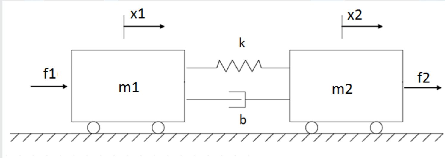
$$\begin{bmatrix} m_1 s^2 + b s + k & -b s - k \\ -b s - k & m_2 s^2 + b s + k \end{bmatrix} \begin{bmatrix} X_1 \\ X_2 \end{bmatrix} = \begin{bmatrix} F_1 \\ F_2 \end{bmatrix}$$
