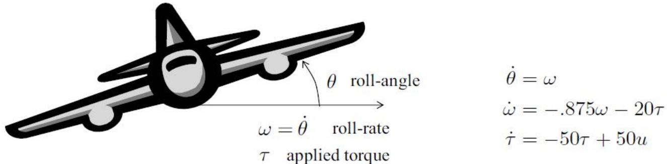
Figure 1.2. Aircraft roll-angle dynamics
