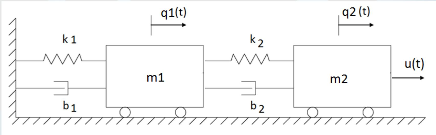
$$\underbrace{\begin{bmatrix} m_1 & 0 \\ 0 & m_2 \end{bmatrix}}_{\mathbf{M}} \begin{bmatrix} \ddot{q}_1 \\ \ddot{q}_2 \end{bmatrix} + \underbrace{\begin{bmatrix} b_1 + b_2 & -b_2 \\ -b_2 & b_2 \end{bmatrix}}_{\mathbf{B}} \begin{bmatrix} \dot{q}_1 \\ \dot{q}_2 \end{bmatrix} + \underbrace{\begin{bmatrix} k_1 + k_2 & -k_2 \\ -k_2 & k_2 \end{bmatrix}}_{\mathbf{K}} \begin{bmatrix} q_1 \\ q_2 \end{bmatrix} = \underbrace{\begin{bmatrix} 0 \\ u \end{bmatrix}}_{\mathbf{F}}$$
