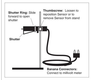
Figure 1 Radiation Sensor
