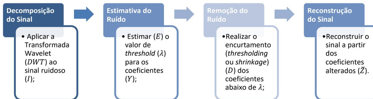
$$\check{Y} = DWT(I) \rightarrow \begin{matrix} \lambda = E(\check{Y}(i)) \\ \check{Z} = D(\check{Y}(i), \lambda) \end{matrix} \rightarrow \hat{I} = IDWT(\check{Z})$$
