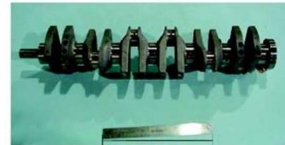
The austempered ductile iron crankshaft for the TVR sports car.
