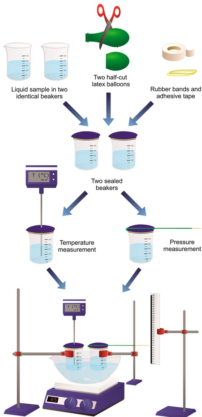
Vapor Pressure Measurement System
