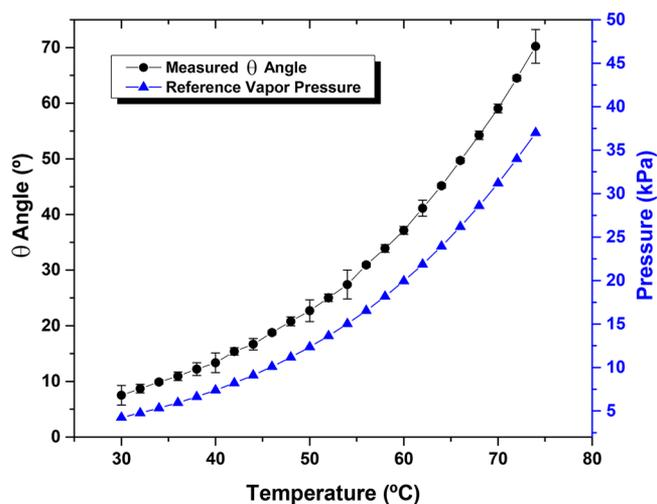
**Figure 3.** Double-y multicurve. The left-hand  $y$ -axis showing the angle as measured by the system, expressed in degrees, for deionized water as a function of temperature ( $^{\circ}\text{C}$ ), which is shown on the  $x$ -axis. Vertical error bars refer to  $\pm 1$  standard deviation ( $n = 3$ ). The right-hand  $y$ -axis shows the reference values for the vapor pressure of water (kPa) as obtained from the data tabulated in the *CRC Handbook of Chemistry and Physics*.<sup>55</sup>
