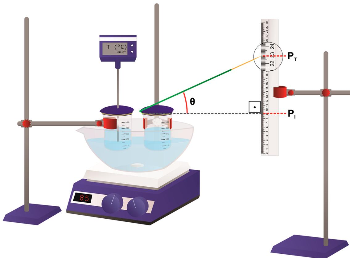
**Figure 2.** Illustration of the assembled system and simulation of the experiment running. The angle measured in the system is shown in detail and is formed because the latex balloon becomes semi-inflated with the pressure exerted by the vapor of the substance in its respective liquid–vapor equilibrium.
