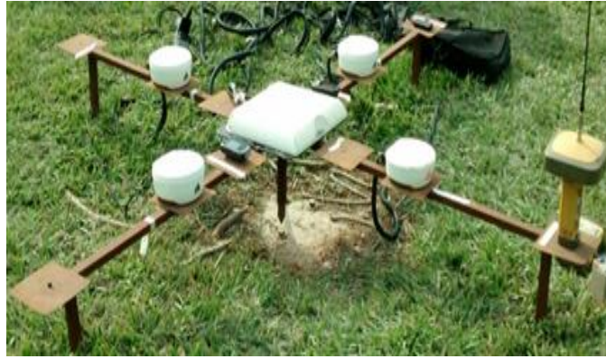
76 FIGURE 1. Supporting frame to allocate GNSS receivers for the static test
