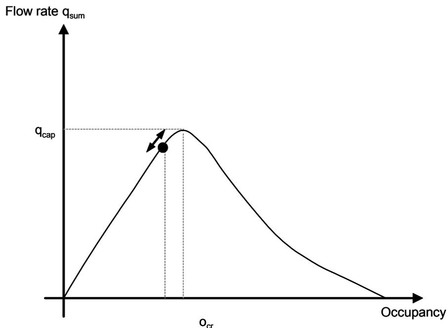
Figure 3.9: Fundamental diagram of free-flow control approach
