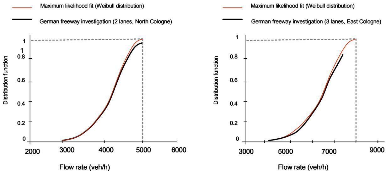
Figure 3.13: Capacity distribution functions for two German freeway sections – 5 min data
