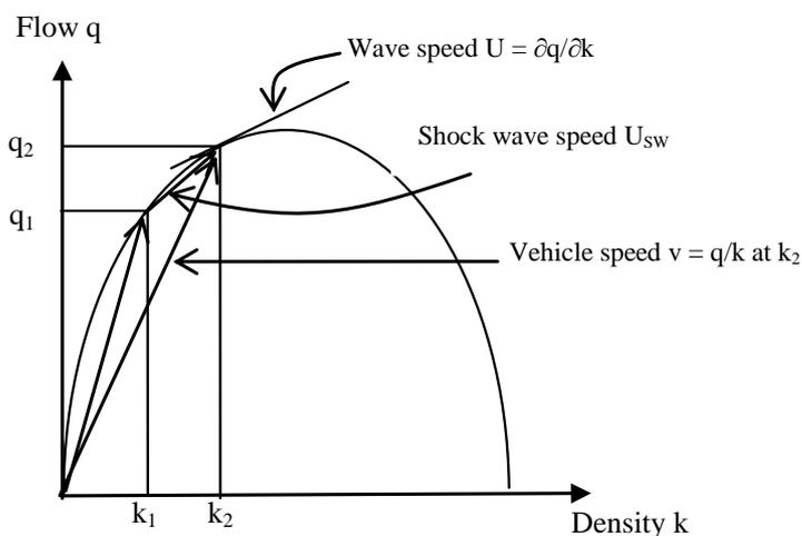
Figure 2.3: The relationship between vehicle speed, wave speed and shock wave speed
