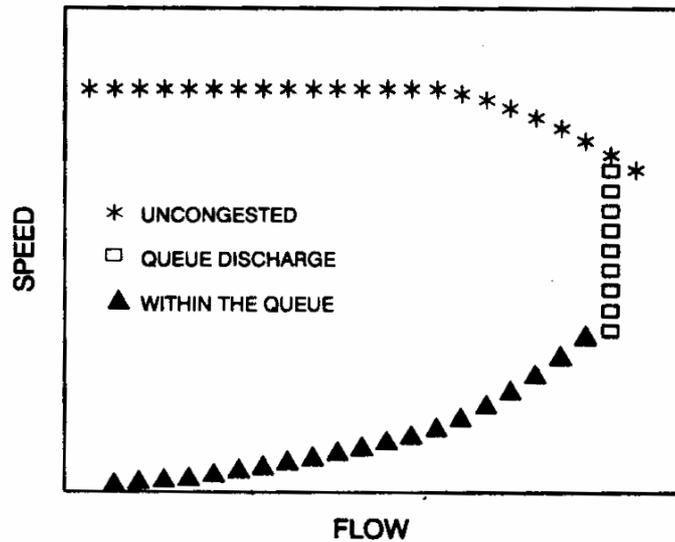
Figure 3.2: Generalised speed flow relation for a typical freeway segment
