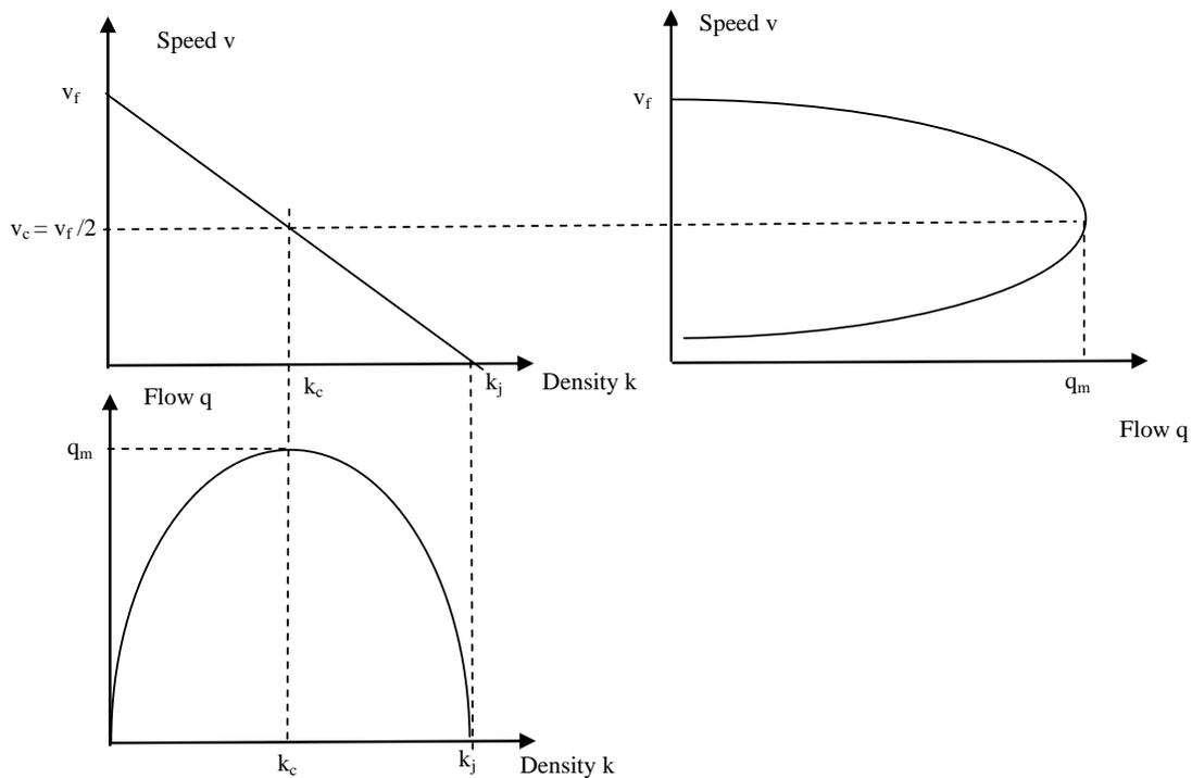
Figure 2.1: Fundamental diagrams assuming linear speed-density relationship
