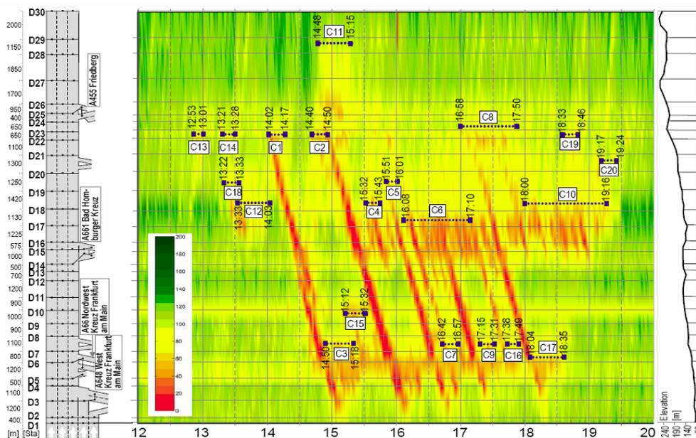
Figure 3.12: A5 speed contour diagram in Lindgren's study – 1 min data
