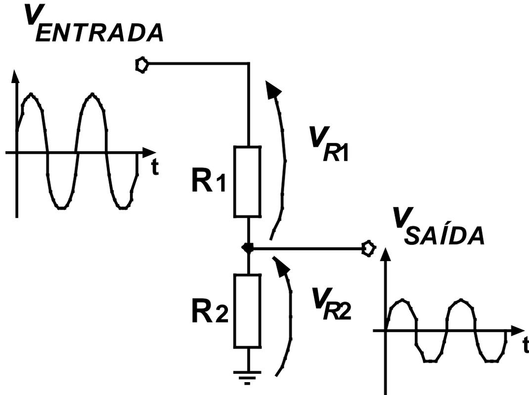
$$V_{SAÍDA} = V_{ENTRADA} * \frac{R_2}{R_1 + R_2}$$
