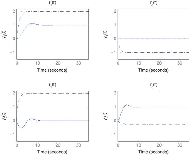
Fig. 4. Step response of the closed loop system after connecting  $C(s)$  in (52) to  $P(s)$  in (45) (solid line), and the step response of the open loop plant  $P(s)$  in (45) (dashed line).
