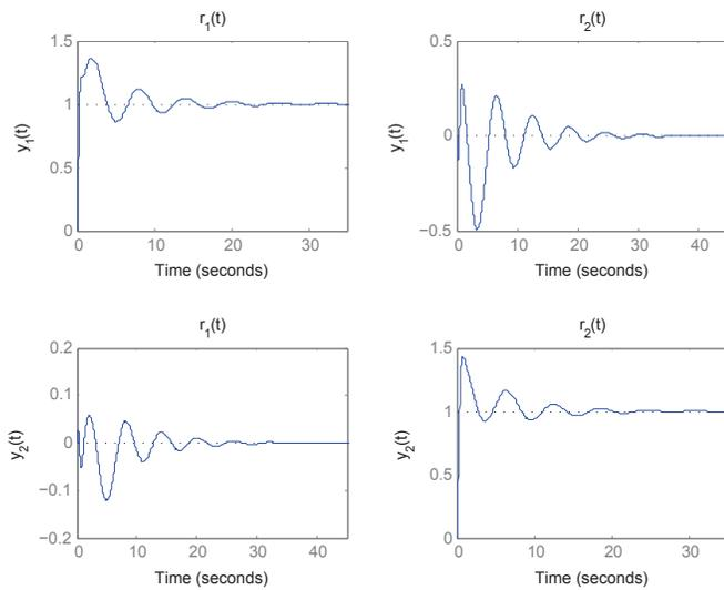
Fig. 5. Step response of the closed loop system after connecting  $C(s)$  in (59) to  $P(s)$  in (54).
