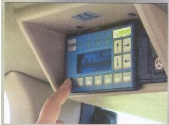
The system components: -mobil Siemens job computer -electro-hydraulically controlled proportional valve -Vehicle terminal controlled in radio box -potentiometer steering unit for the left armrest -sensor bar with four ultrasonic sensors for the front hitch
