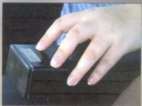
An optional feature is the small potentiometer steering wheel, mounted on the left hand armrest. With this feature the driver can do quick and easy headland turns. He just switches from automatic steering to potentiometer steering and he can turn with a comfortable small control wheel on his armrest.
