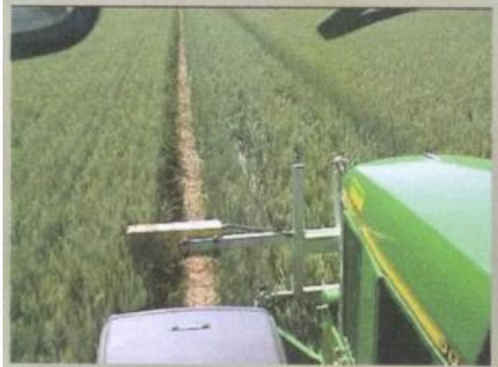
The Ultrasonic sensing bar mounted at the front hitch, recognizes differences greater than 10 cm on the field and transforms this into steering signals via a small integrated valve in the steering circuit.
