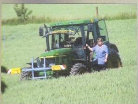
The system turns off and back to normal manual controlled steering as soon as: -the steering wheel is turned -23-km/h limit is exceeded -the cab doors are opened -failures of system components -main switch is switched off -main menu is being quit
