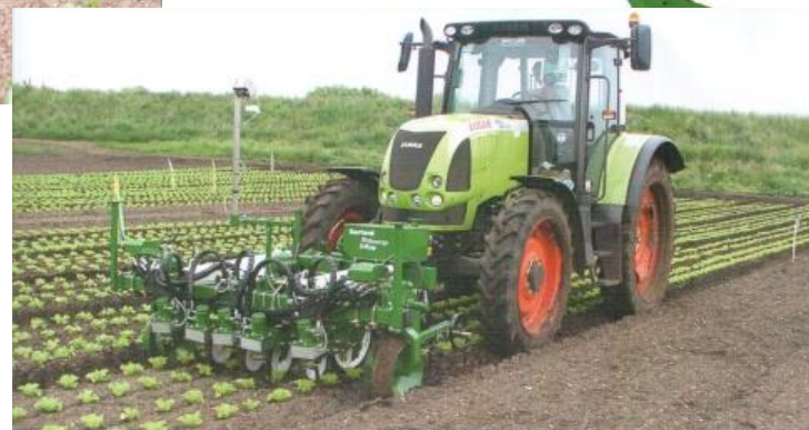
Smaller single bed Robocrop InRow Weeders utilise a single camera.
