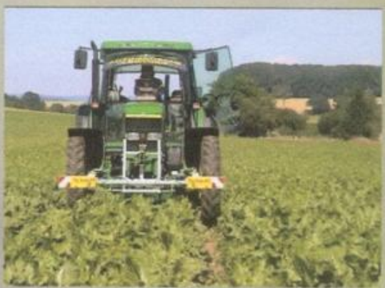
The driver can rely on the tractor automatically following the rows. He can concentrate on the application, control and optimize the output to save products and money while improving crop quality. Late evening and night spray application with limited visibility is no longer a problem.
