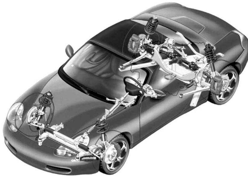
Fig. 8.1-46 The Porsche Boxster (1996) has a water-cooled engine which is longitudinally installed in front of the rear axle. The front axle is designed as a spring strut-type axle. The transverse link is arranged almost in extension of the wheel axle; it is connected to the longitudinal link by a strut bush which is soft for reasons of comfort. This open design and link geometry make it possible to combine a high level of driving precision, a result of rigid wheel control, with riding comfort, owing to the longitudinal elasticity of the axle. At a camber angle of 8^\circ , good straight running results from the large castor displacement of 41 mm. The kingpin offset is -7 mm and the disturbing force lever arm is 83 mm. The pitch centre of the front axle was located near to the road to achieve kinematic wheel recession of the axle, which is important for riding comfort, with the result that braking-torque compensation is only 10%. The rear axle is also a spring strut-type axle in an open link design; the wheel carrier, hub and bushes as well as the transverse link are the same as those found on the front axle. The open design makes it possible to have an inwardly inclined elastokinematic axis of rotation, so that a stabilizing toe-in position of the rear wheels is produced during braking. The axle can also be designed to understeer when subject to lateral forces. The main disadvantages of the mid-engine design are apparent from the boot space: only 130 l are available at both the front and back.
