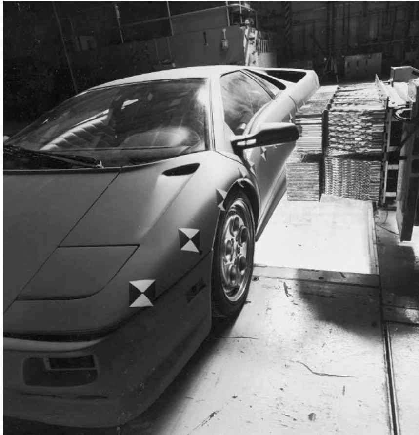
Fig. 17.1-4 This aluminium honeycomb used in a side impact test is profiled to represent the vertically varying stiffnesses of the other car.
