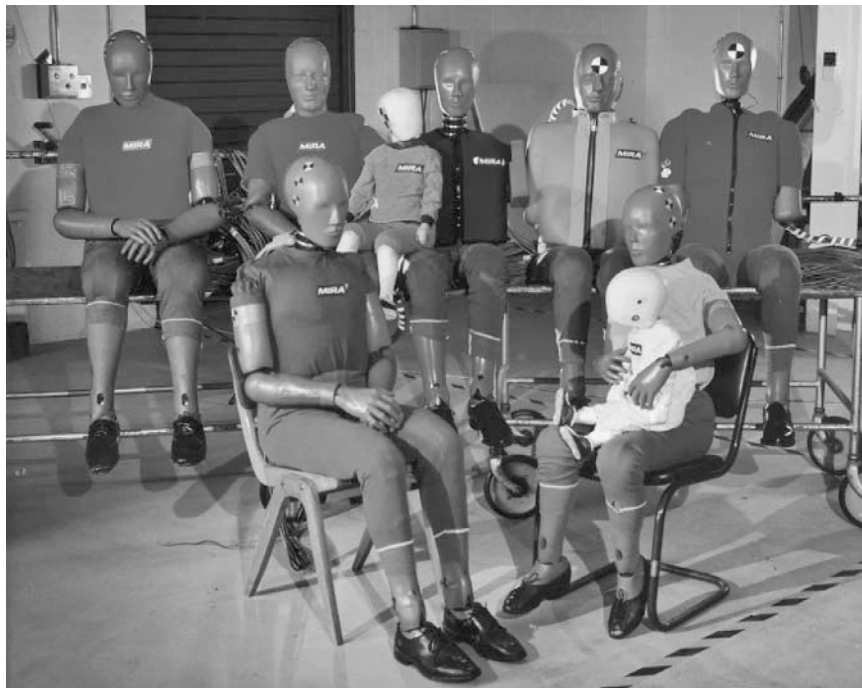
Fig. 17.1-8 A range of male and female child and adult Anthropomorphic Test Devices (ATVs) ranging in weight up to 14 stone (90 kg) is used by MIRA.
