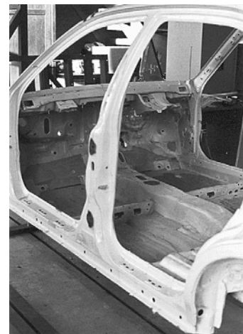
Fig. 16.1-24 Integral body floor assembly, showing structural members.
