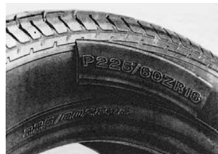
Fig. 10.1-17 ZR tyres manufactured specially for the American market and marked with a 'P' do not meet the European standard and are therefore not authorized here (photograph: Dunlop factory).
