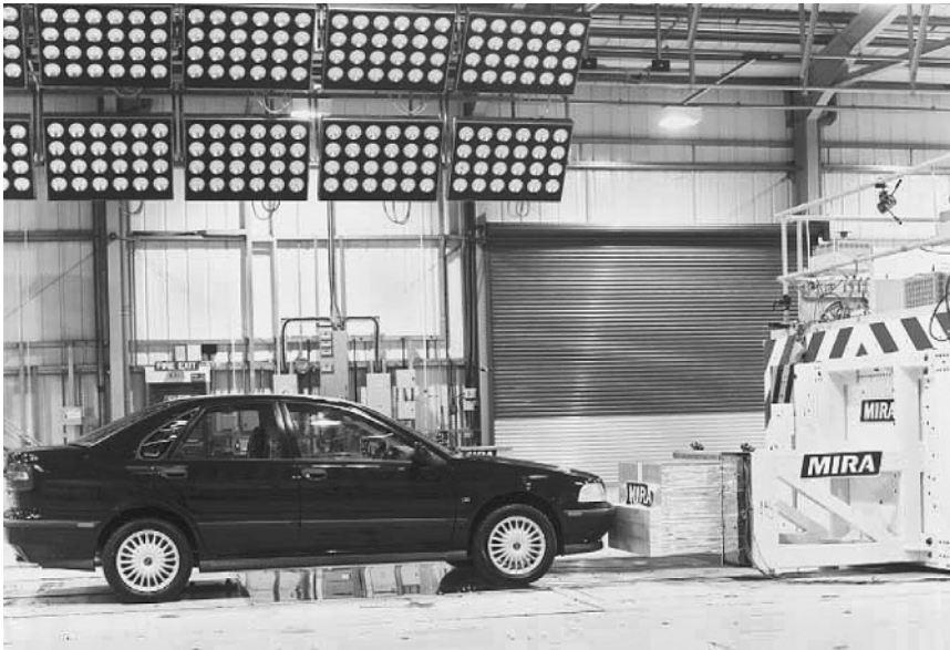
Fig. 17.1-3 Here a dummy front end of a car represented by an aluminium honeycomb structure is fixed to the concrete block to simulate the crushing of the other car involved in the front end impact.
