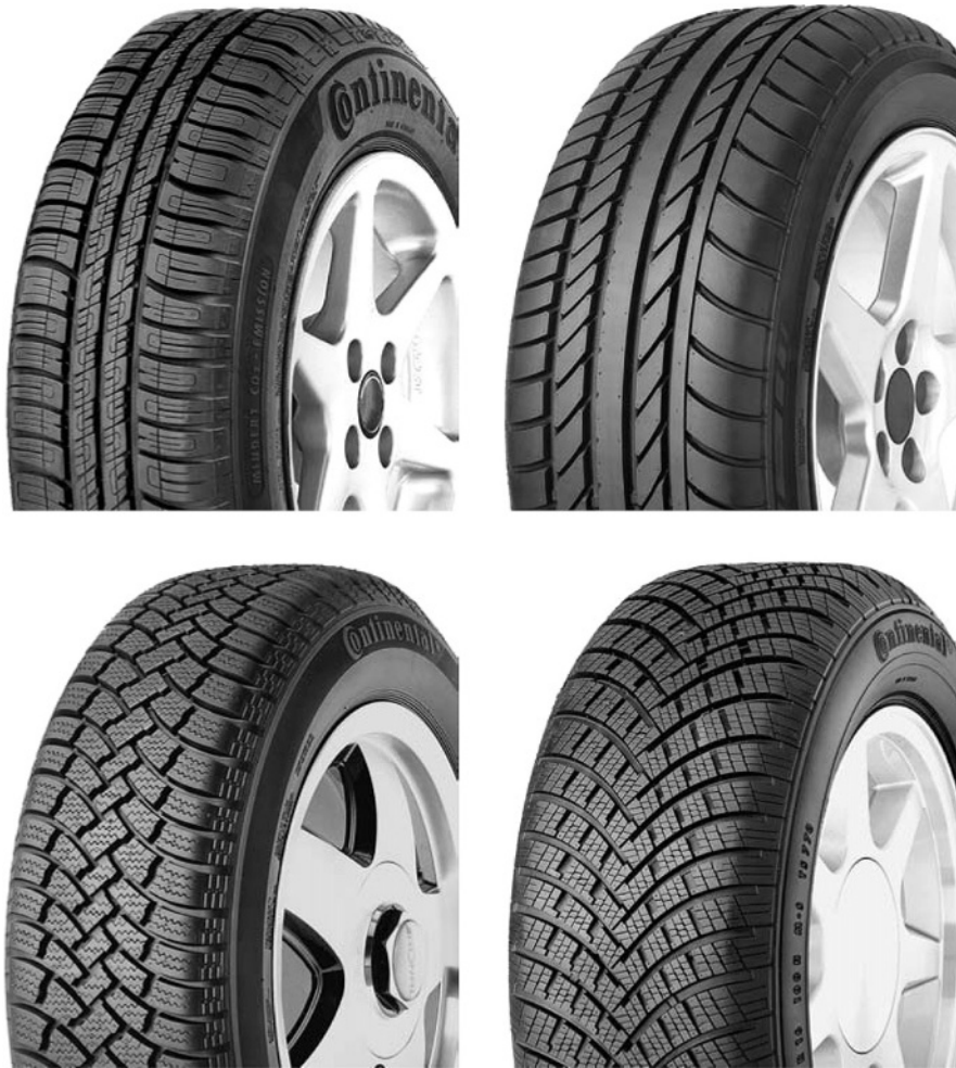
Fig. 10.1-19 Designs of Continental tyre. (Top) Summer tyre (tyre foot prints, see Fig. 10.1-9) EcoContact EP (size 185/65 R14T) and Sport Contact (size 205/55 R16W). (Below) Winter tyre WinterContact TS760 (size 185/65 R14T) and WinterContact TS770 (size 235/60 R16H).
