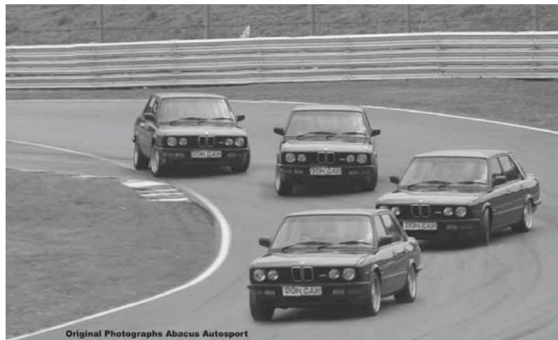
Fig. 15.1-45 Driver and vehicle behaviour for a post-limit turn-in event (photograph courtesy of Don Palmer, www.donpalmer.co.uk ).
