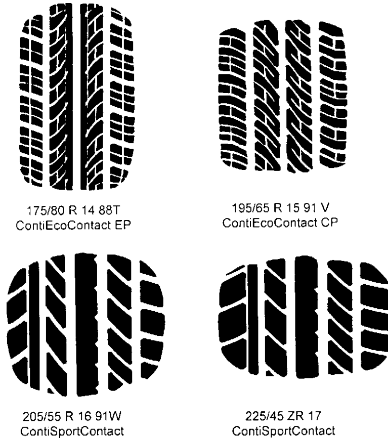
Fig. 10.1-9 If they have the same outside diameter and load capacity the four tyre sizes used on medium-sized passenger cars are interchangeable. The series 65, 55 and 45 wide tyres each allow a 1" larger rim (and therefore larger brake discs). The different widths and lengths of the tyre contact patch, known as 'tyre print', are clearly shown (Fig. 10.1-19), as are the different designs of the standard road profile and the asymmetric design of the sports profile (see also Section 10.1.2.10). The 65 series is intended for commercial vehicles, and the 60, 55 and 45 series for sports cars. (Illustration: Continental; see also Fig. 10.1-19.)
