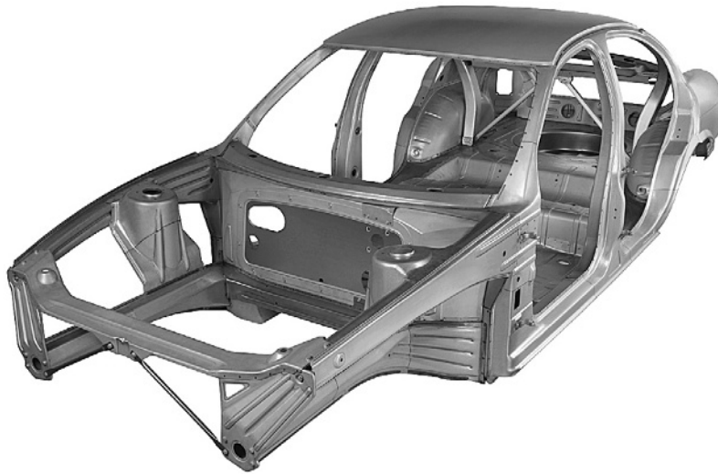
Fig. 16.1-25 The ultralight steel auto body (ULSAB) (courtesy of the ULSAB consortium).
