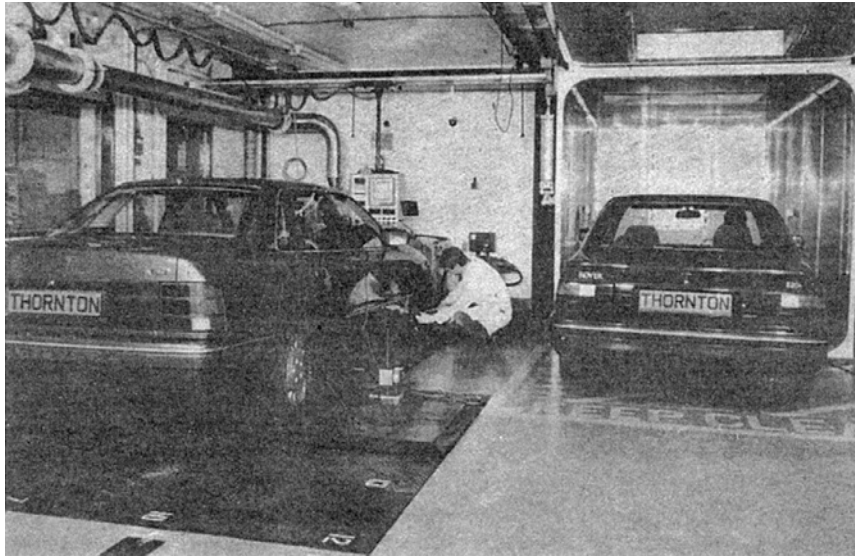
Fig. 3.1-6 (Left) Sealed Housing for Evaporative Determination (SHED) installed alongside a chassis dynamometer (right) in a thermostatically controlled chamber at the Shell Thornton Research laboratories.
