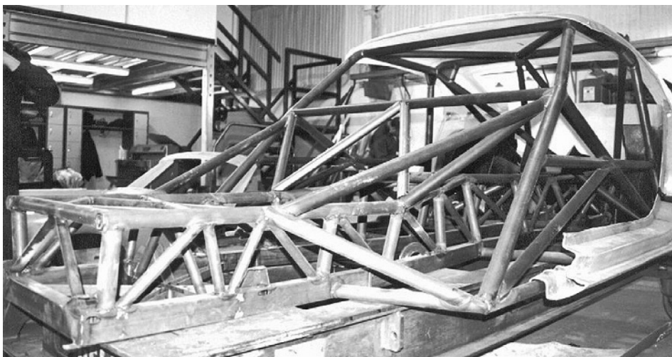
Fig. 16.1-17 Triangulated sports car structure with integrated roll cage (Roots et al. 1995 with original permission from TVR Ltd).
