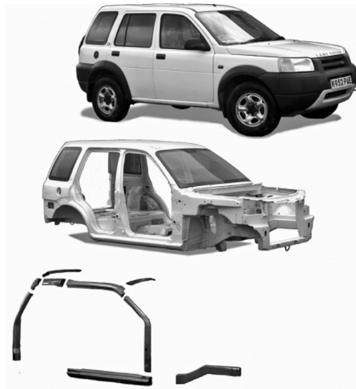
Fig. 18.1-34 Freelander design in steel and proposed alternative hydroformed parts. 16
