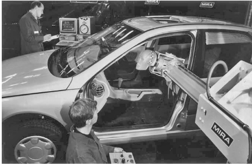
Fig. 17.1-10 The Head Impact Test System (HITS) rig used by MIRA for assessing the occupant-friendliness of interior components and trim.
