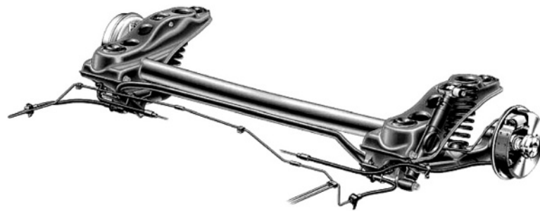
Fig. 8.1-13 Trailing-arm rear suspension of the Mercedes-Benz A class (1997). In order to minimize the amount of room required, the coil spring and monotube gas-pressure shock absorber are directly supported by the chassis subframe. The connecting tube is stress optimized oval shaped in order to withstand the high bending moments from longitudinal and lateral wheel forces which occur in the course of driving. The torsion-bar stabilizer proceeds directly from the shock-absorber attachment for reasons of weight and ease of assembly. When establishing the spring/shock-absorber properties, the line along which the forces act and which is altered by the lift of the wheel is to be taken into consideration, as a disadvantageous load-path can occur with jounce. The two front subframes are hydraulically damped in order to achieve a good level of comfort (hydromounts). The chassis subframe can make minor elastokinematic control movements. When designing subframe mounts, it is necessary to ensure that they retain their defined properties with regard to strength and geometry even with unfavourable conditions of use (e.g. low temperatures) and for a sufficiently long period of time, because variations in the configuration have a direct effect on vehicle performance. The longitudinal arms which run on tapered-roller bearings and which are subject to both flexural as well as torsional stress are designed in the form of a parallelogram linkage. In this way, the inherent disadvantage of a trailing arm axle – unwanted toe-in as a result of the deformation of the link when subject to a lateral force – is reduced by 75%, according to works specifications.
