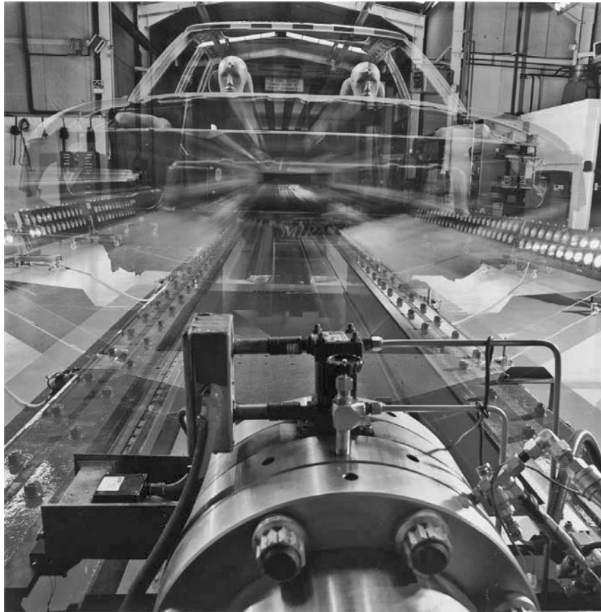
Fig. 17.1-6 In the MIRA impact simulation laboratory, what is in effect a giant air gun projects the sled at speeds of up to 56 miles per hour towards its target.
