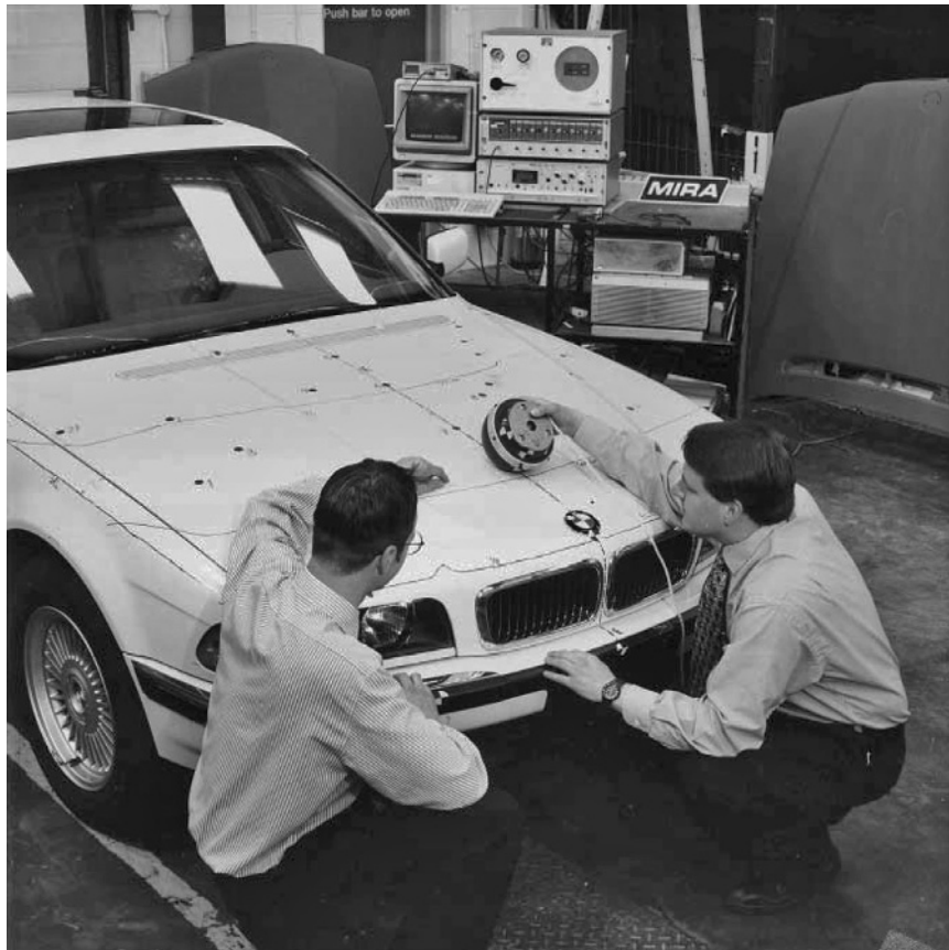
Fig. 17.1-9 Experts assessing the performance of a BMW bonnet when struck by a fully instrumented dummy head.
