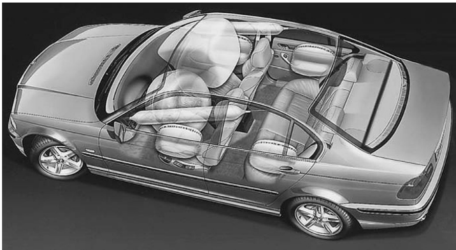
Fig. 9.1-25 BMW passenger car with air bags for the front, sides and head (front and back).
