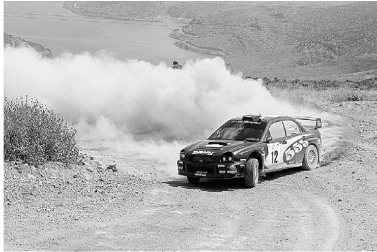
Fig. 15.1-47 Large body slip angles are unavailable to normal drivers except as part of an accident. Subaru WRC, Greece 2002 (courtesy of Prodrive).
