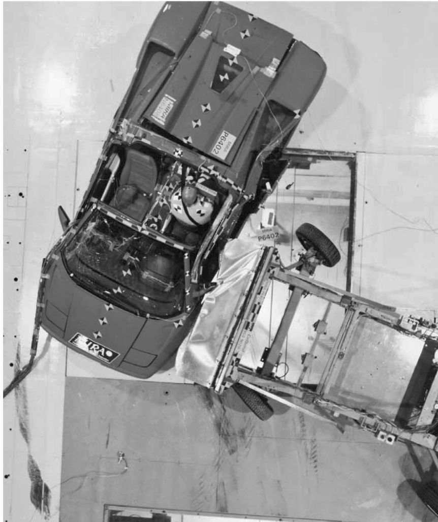
Fig. 17.1-5 View from above of an impact test in which a sled, on which is mounted a dummy front end, is propelled towards the side of the target vehicle.
