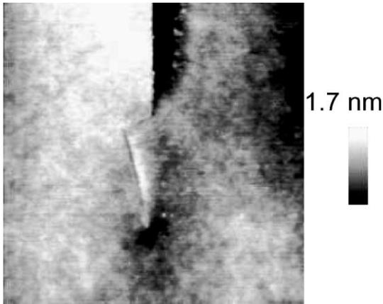
Fig. 9. Direct AFM evidence of the non-coplanar repropagation of an aged indentation crack. Top view, size of field:  $20\ \mu\text{m} \times 2\ \mu\text{m}$  (from [20]).
