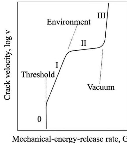
Fig. 1. Velocity of a running crack versus strain energy release rate: general features (from [25]).
