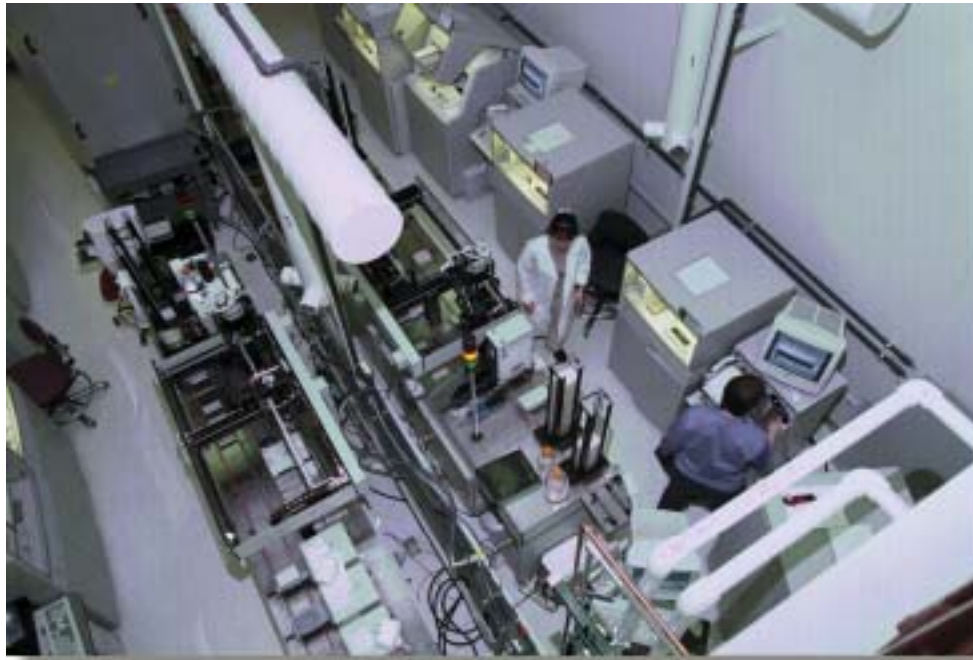
Figure 12-3 Part of the automated production line of a major human genome sequencing center. All this equipment is used for rapid processing of huge numbers of clones for DNA sequencing. [©Bethany Versoy; all rights reserved.]
