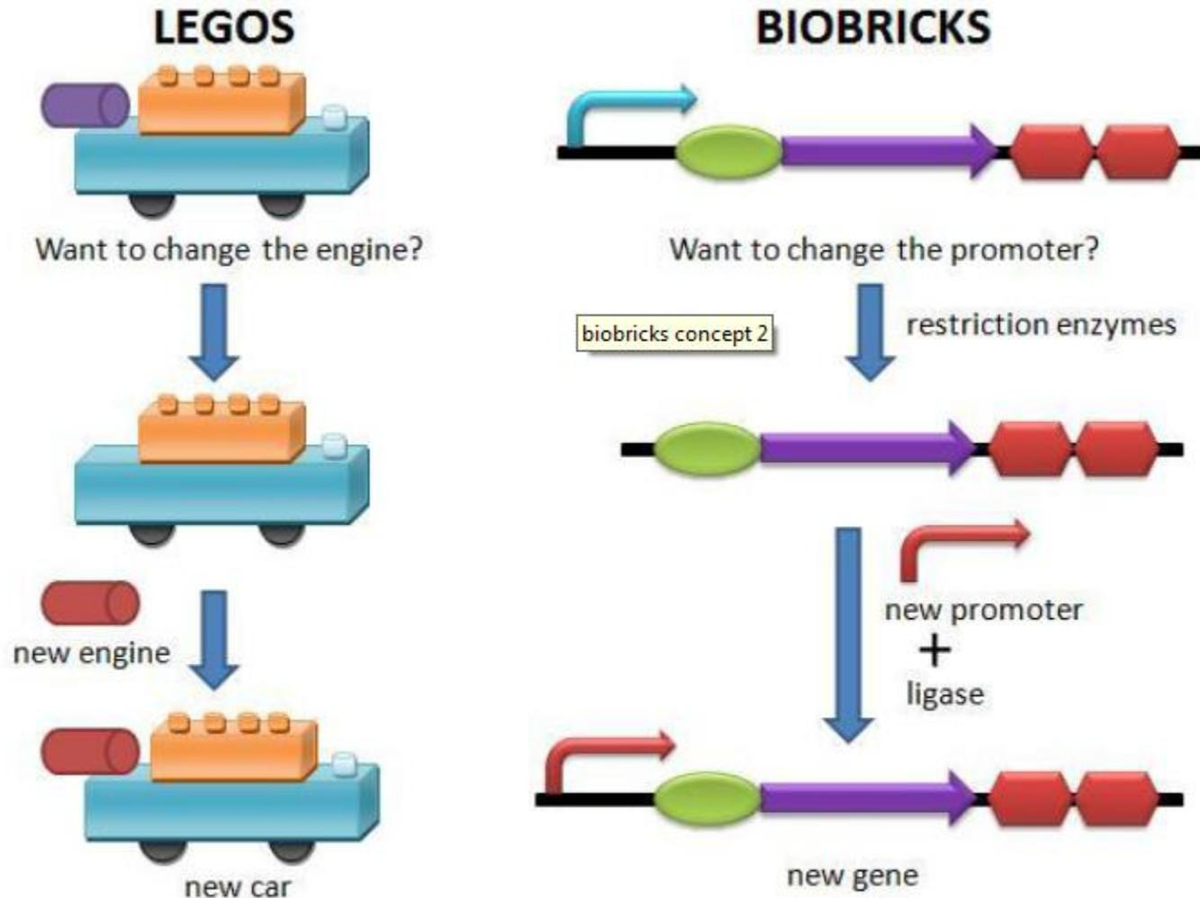
Figure2: The concept of interchangeable parts in biobricks
