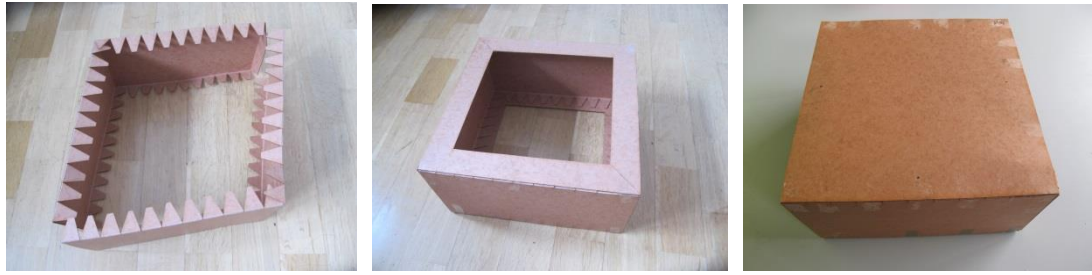
Figure 4.4. 6 Improvement of construction details for the cellular structure
