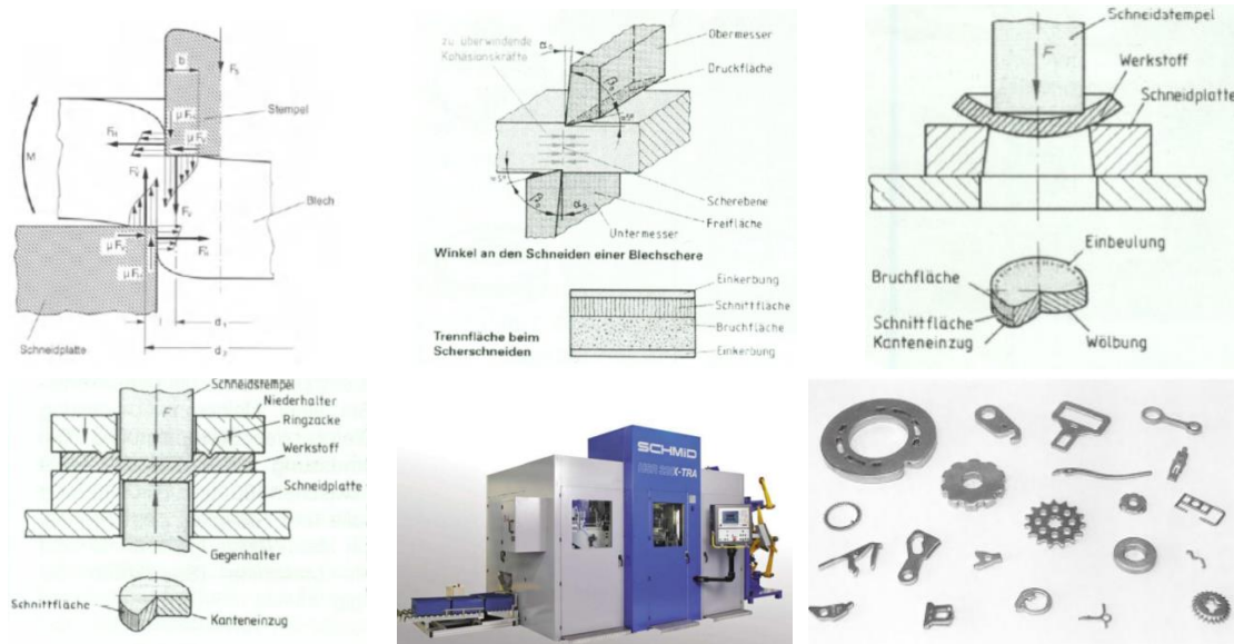
Figure 3.3.3 Traditional shear cutting techniques (König & Klocke, 1990)
