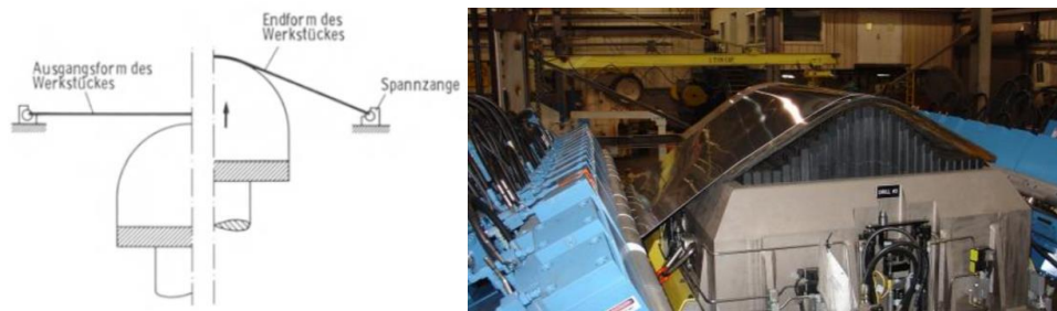
Figure 3.3.8 Tensile Forming techniques (König & Klocke, 1990)
