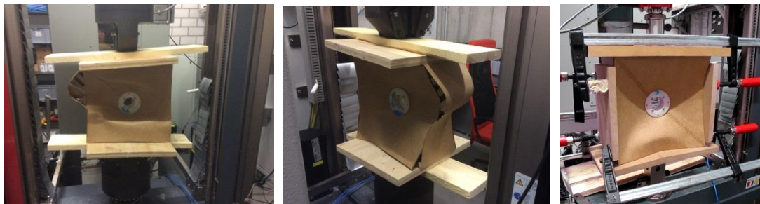
Figure 4.4. 5 Deformations in the pre-tests
