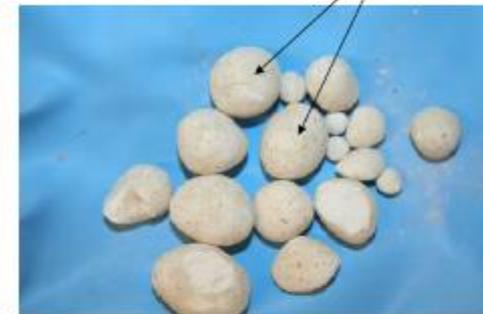
Lime at 100% lignin firing (Sample K32)
