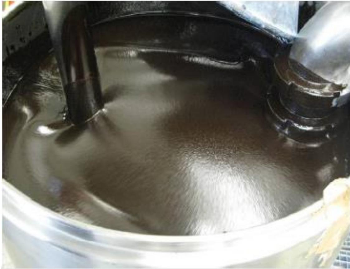
We have also successfully mixed lignin with glycerine (from bio-diesel production) and also with the tar oil from refining of crude tall-oil
