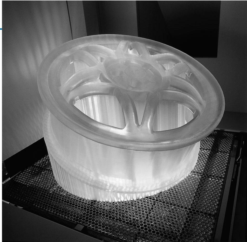
A part produced by stereolithography (photo courtesy of 3D Systems, Inc.).
