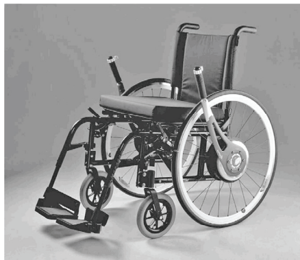
Fig. 6. Lever propulsion system (Requejo et al., 2008)
