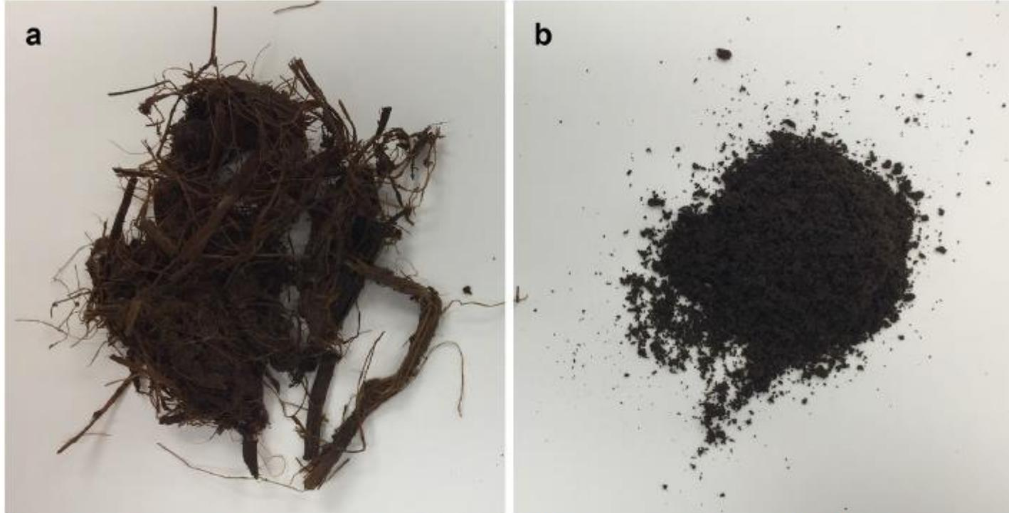
**Fig. 6** Size reduction of dilute acid-pretreated corn stover by disk milling. **a** Dilute acid-pretreated sample; **b** dilute acid-pretreated and disk-milled sample
