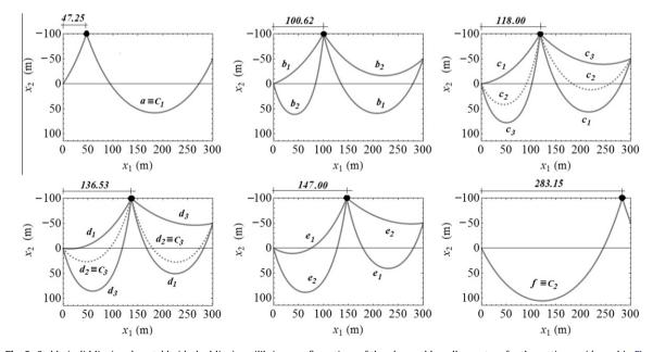
Fig. 8. Stable (solid line) and unstable (dashed line) equilibrium configurations of the plane cable pulley system for the settings evidenced in Fig. 6.
