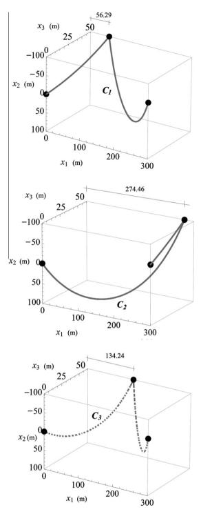
Fig. 9. Equilibrium positions of cable with pulley in spatial configuration.
