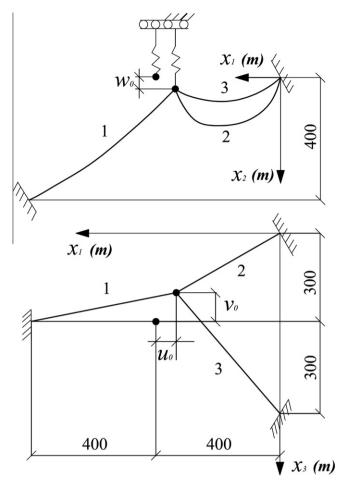
Fig. 4. Cable system with a spring.
