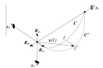
**Fig. 1.** Unstrained configuration *C* and stretched configuration *C*<sup>\*</sup> under uniformly distributed load.
