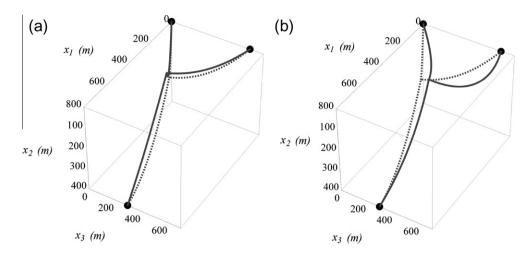
Fig. 5. Unstrained (dotted line) and stretched (solid line) configuration of the cable system with a spring: (a) without wind force; (b) with wind force.
