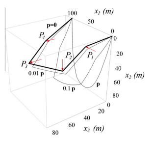
**Fig. 3.** Deformed shape of a cable under a uniformly distributed vertical load **p**, 0.1**p**, 0.01**p**, 0.001 **p** and four point forces (gray lines) compared with the funicular of point forces, i.e. the deformed shape for  $\mathbf{p} = \mathbf{0}$  (black line).
