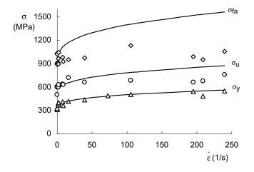
Various stress predictions for the steel alloy BS EN 10025 FE430A according to the Cowper—Symonds equation, with its constants determined from the yielding stress.
