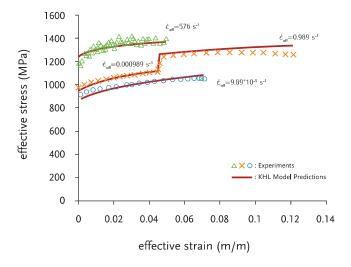
Titanium alloy Ti-6Al-4V compressive stress—strain behaviour at various strain rates. Adapted from Experimental and numerical analysis of high strain rate response of Ti-6Al-4V titanium alloy A.Bragov, A. Konstantinov, A. Lomunov, I.Sergeichev and B. Fedulov, DYMAT 2009, p. 1465–1470, 2009.
