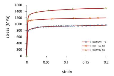
A titanium alloy mechanical behaviour at various strain rates.
