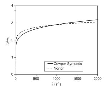
Predicted dynamic flow stress for a typical mild steel. Continuous line, Cowper—Symonds equation with p=5 and  $D=40/\mathrm{s}$ . Dashed line, Norton equation with  $\dot{\varepsilon}_0=0.001/\mathrm{s}$  and q=0.077. In both predictions  $\sigma_0=235$  MPa.
