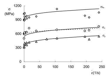
Prediction of the constitutive law  $\sigma_{eq_d}=\sigma_{eq_s}+\bar{m}\dot{\varepsilon}^{\bar{n}}$  for steel alloy BS EN 10025 FE430A together with experimental results for  $\Delta$ : lower yield,  $\sigma_y$ ,  $\circ$ : ultimate,  $\sigma_u$ , and  $\diamond$ : failure,  $\sigma_{fa}$ , stresses versus strain rate.
