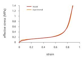
A polymer stress—strain behaviour and the corresponding model prediction.
