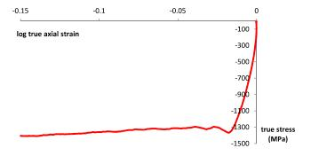
The behaviour of a titanium alloy at a strain rate of 1000/s.
