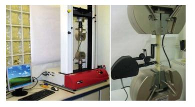
A remark is that tensile test machines have also an accurate sensor to measure the jaw displacement. However, this information needs to be handled with care since the machine transverse beam, which holds the jaws, deforms as the stretching load increases. This adds to the actual strain value experimented by the specimen. Hence, a local displacement measure, as the one yielded by strain or clip gauges, is far better to be used for the calculation of the strains.
