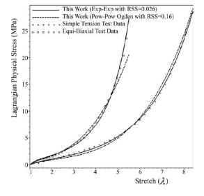
Stress—strain curve for a polymer showing non–linear behaviour at an early stage of loading (from H. Darijani, R. Naghdabadi and M.H. Kargarnovin, Constitutive modeling of rubberlike materials based on consistent strain energy density functions, Polymer Engineering and Science, p. 1058–1066, 2010).
