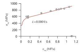
Stress-strain curves in the engineering and true equivalent spaces for the same ductile steel alloy.
