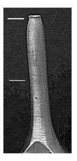
Necking zone in a tensile specimen and a sketch of the stress field.
