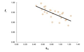
The factor  $f_c$  for a ductile steel alloy.
