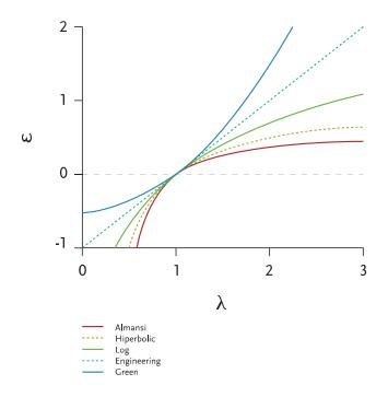
Different strain measures as a function of the stretching.
