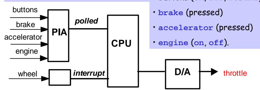
Wheel revolution sensor generates interrupts to enable the car speed to be calculated.
