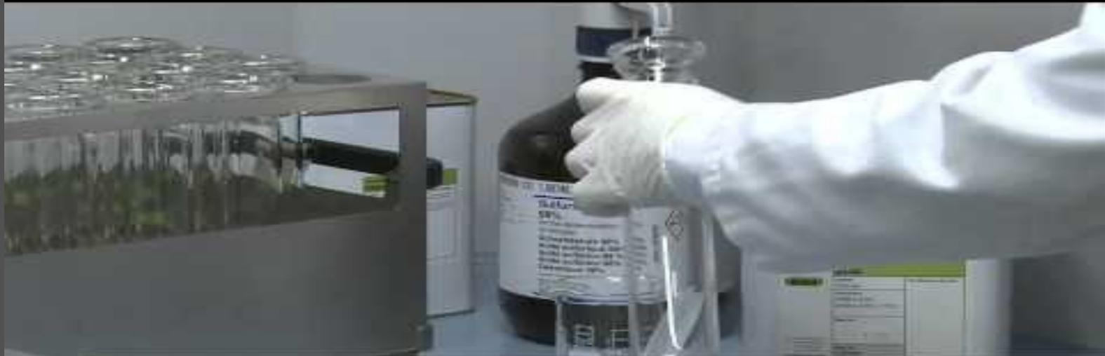
Add the BUCHI Kjeldahl Tablets and the corresponding volume of sulfuric acid
