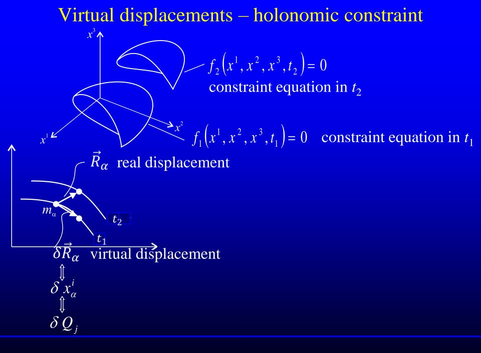
• Virtual displacements are kinematically admissible displacements in a fixed time  $\underline{t}$ , that is, satisfy the constraint equations for that time  $\underline{t}$ .
