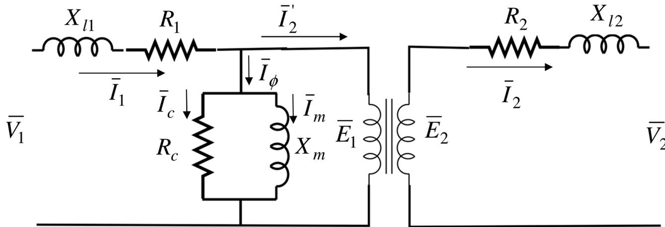
$$P_{Cu} = I_1^2 R_1 + I_2^2 R_2 = I_1^2 R_{eq,1} = I_2^2 R_{eq,2}$$
