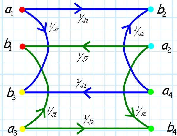
It is evident that, just as with the directional coupler, the ports are **matched** and the device is **lossless**. Note also, that if a signal is incident on one port only, then there will be a port from which **no** power will exit (i.e., an **isolation** port).
