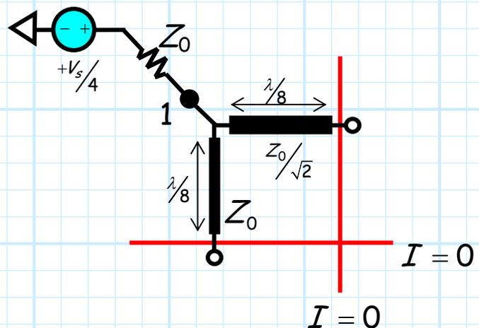
The circuit has simplified to a 1-port device consisting of the parallel combination of two  $\lambda/8$  open-circuited stubs. The admittance of a  $\lambda/8$  open-circuit stub is:
