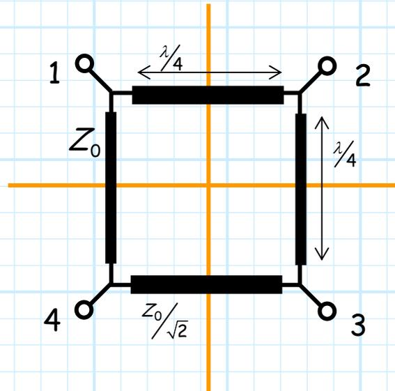
To determine the scattering parameters  $S_{11}, S_{21}, S_{31}, S_{41}$ , of this network, a matched source is placed on port 1, while matched loads terminate the other 3 ports.
