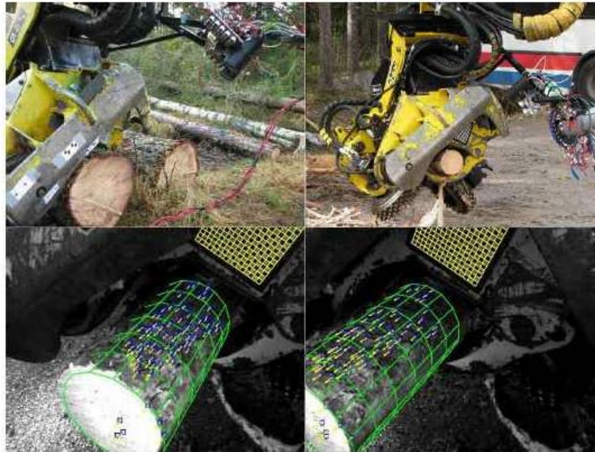
Fig. 5 Harvester head with stereo camera pairs and lights attached (above). Left and right stereo images showing selected features, trunk estimate and the tracked chessboard pattern.
