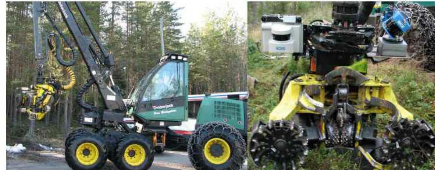
Fig. 1 Timberjack 1070 harvester with John Deere 745 head on test site on the left and standing tree measurement sensors attached to a 745 head on the right.
