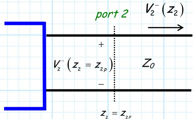
The complex ratio between  $V_1^+(z_1 = z_{1p})$  and  $V_2^-(z_2 = z_{2p})$  is known as the **scattering parameter  $S_{21}$** :
