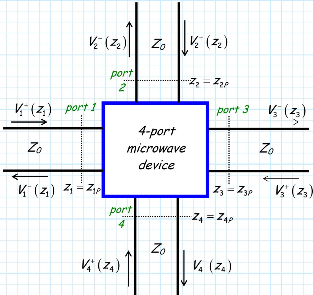
Note that we have now characterized transmission line activity in terms of incident and "reflected" waves. Note the negative going "reflected" waves can be viewed as the waves **exiting** the multi-port network or device.
