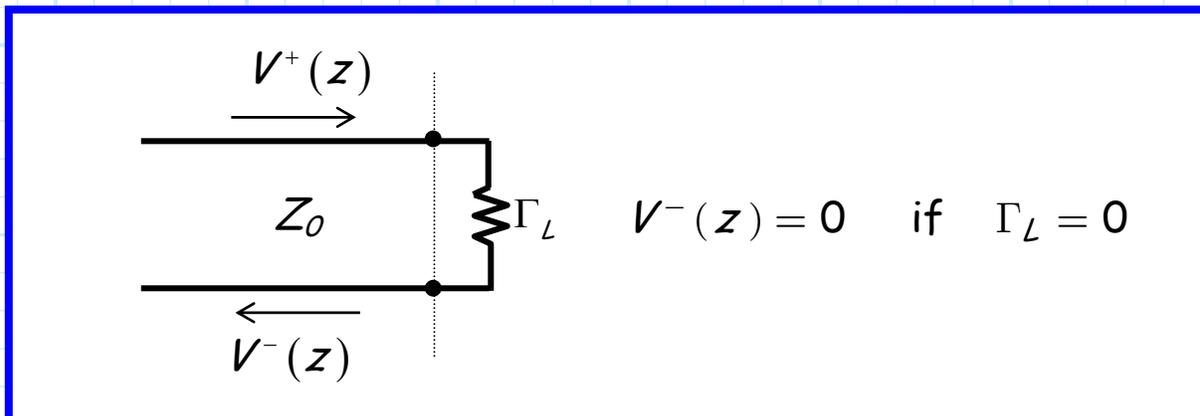
In this original case, the wave **incident** on the load is  $V^+(z)$  (**plus** direction), while the **reflected** wave is  $V^-(z)$  (**minus** direction).
