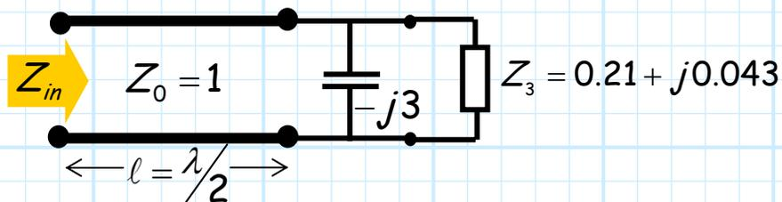
Now we find that the impedance  $Z_3$  is **parallel** to the capacitor. We can **combine** the two impedances and define the result as impedance  $Z_4$ :
