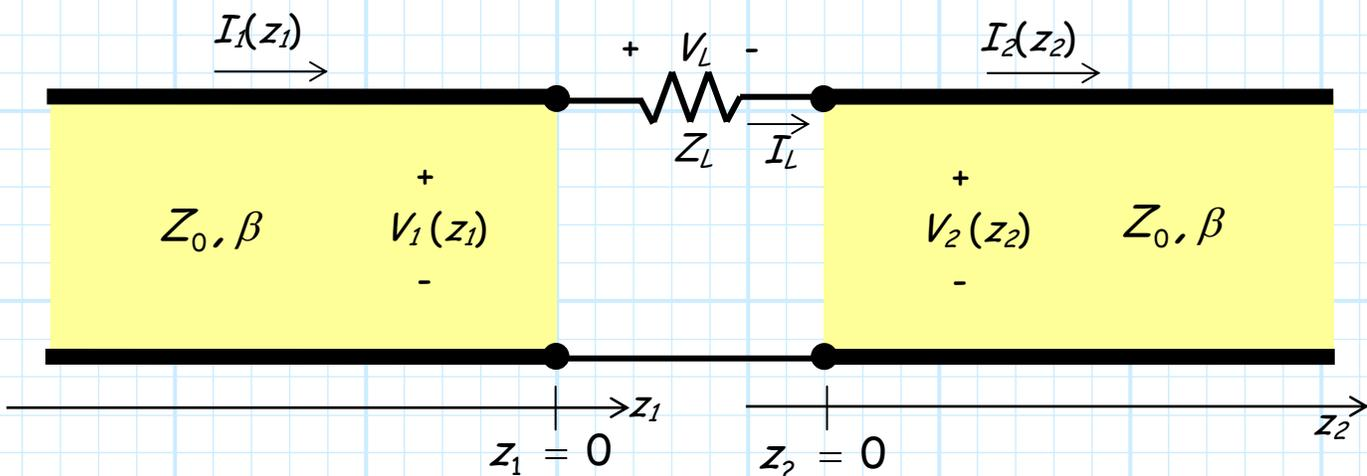
I.E., Two transmissions of **identical** characteristic impedance are connect by a **series** impedance  $Z_L$ . This second line is eventually **terminated** with a load  $Z_L = Z_0$  (i.e., the second line is **matched**).
