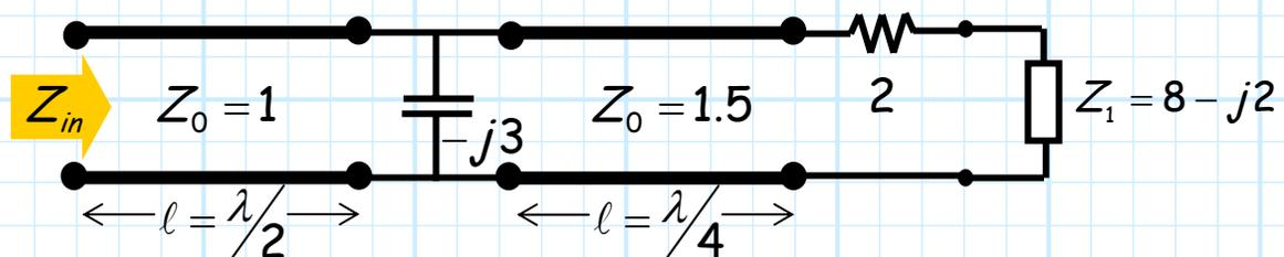
Note the resistor is in **series** with impedance  $Z_1$ . We can **combine** these two into one impedance defined as  $Z_2$ :
