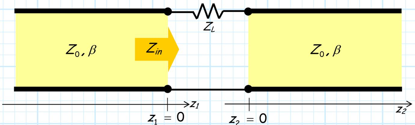
Note that since the second line is (eventually) terminated in a matched load, the input impedance at the **beginning** of the **second** line is simply equal to  $Z_0$ .
