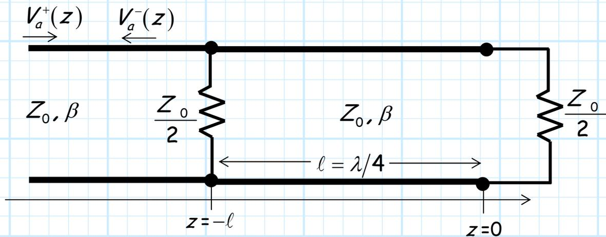
Specifically, we can determine the input impedance of this circuit:
