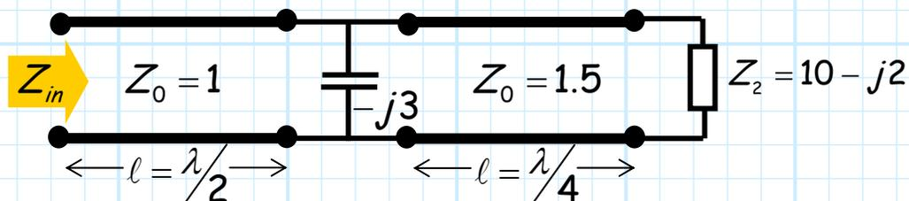
Now let's define the input impedance of the **middle** transmission line section as  $Z_3$ :
