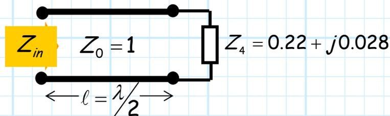
Note that the remaining transmission line section is a **half wavelength!** This is one of the **special** situations we discussed in a previous handout. Recall that the **input** impedance in this case is simply equal to the **load** impedance:
