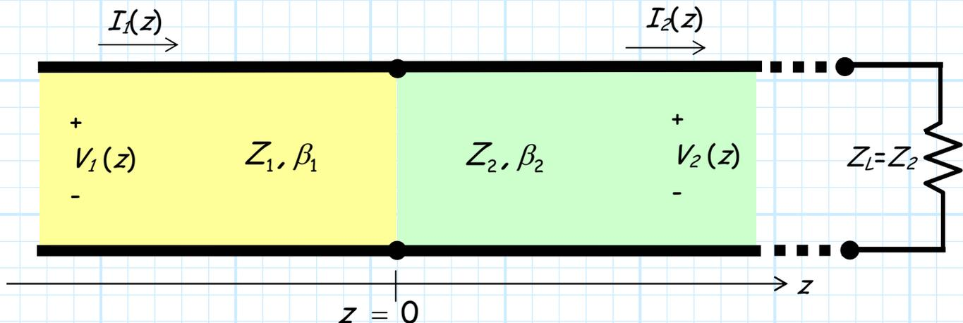
I.E., a transmission line with characteristic impedance  $Z_1$  **transitions** to a **different** transmission line at location  $z=0$ . This second transmission line has different **characteristic impedance**  $Z_2$  ( $Z_1 \neq Z_2$ ). This second line is **terminated** with a load  $Z_L = Z_2$  (i.e., the second line is **matched**).
