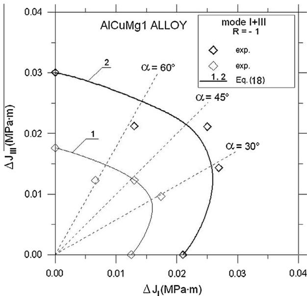
Fig. 13. Comparison between experimental results for different bending to torsion ratios and those calculated according to Eq. (28) for AlCuMg1 alloy.
