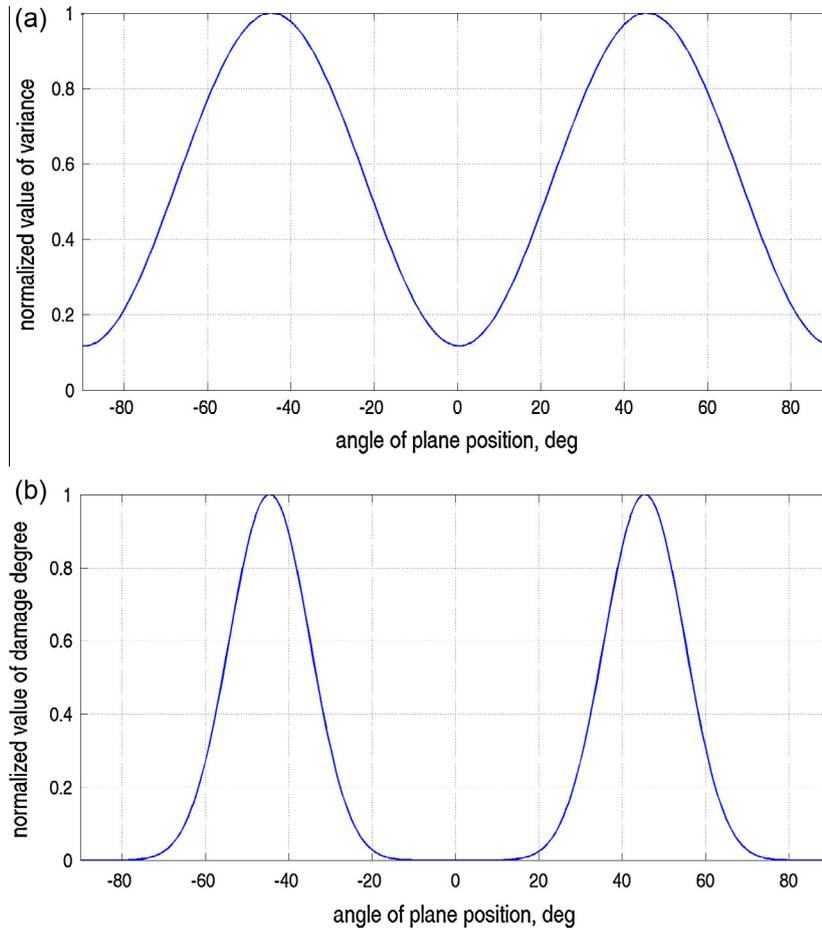
Fig. 4. Dependence of the normalized value of: (a) variance and (b) damage accumulation on the angle  $\xi$  of critical plane position.
