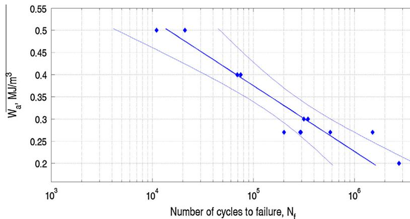
Fig. 8. The energy fatigue characteristic for C45 steel.
