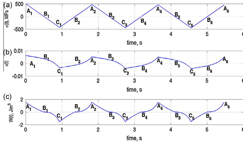
Fig. 7. Example of: stress courses (a), strain courses (b), energy parameter courses (c) for test with controlled strain energy density amplitude  $W_a$  (Eq. (27)).
