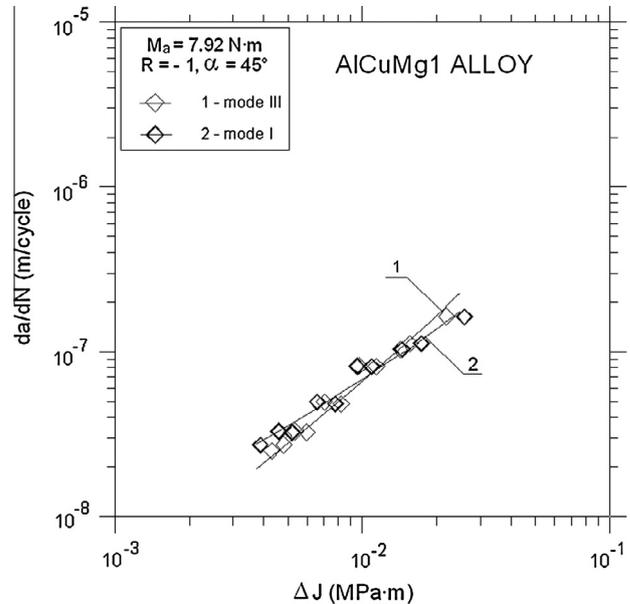
Fig. 14. Fatigue crack growth rate  $da/dN$  versus  $\Delta J$ , for AlCuMg1 alloy and  $\alpha = 45^\circ$ .
