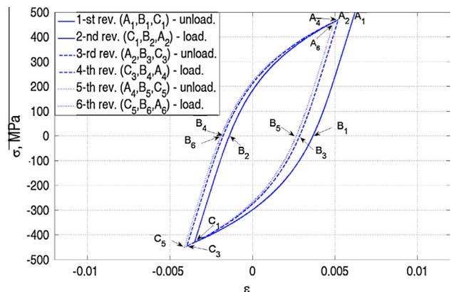
Fig. 6. Example of hysteresis loops ( $\sigma$ - $\varepsilon$ ) for test with strain energy density amplitude  $W_a$  controlled (Eq. (27)).
