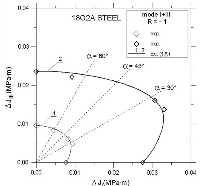
Fig. 11. Comparison between experimental results for different bending to torsion ratios and those calculated according to Eq. (28) for 18G2A steel.
