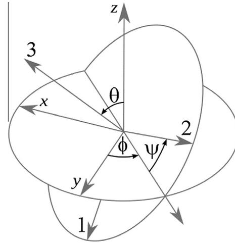
Fig. 3. Description of principal stress directions 1, 2, 3 through the Euler angles  $\phi, \theta, \psi$ .
