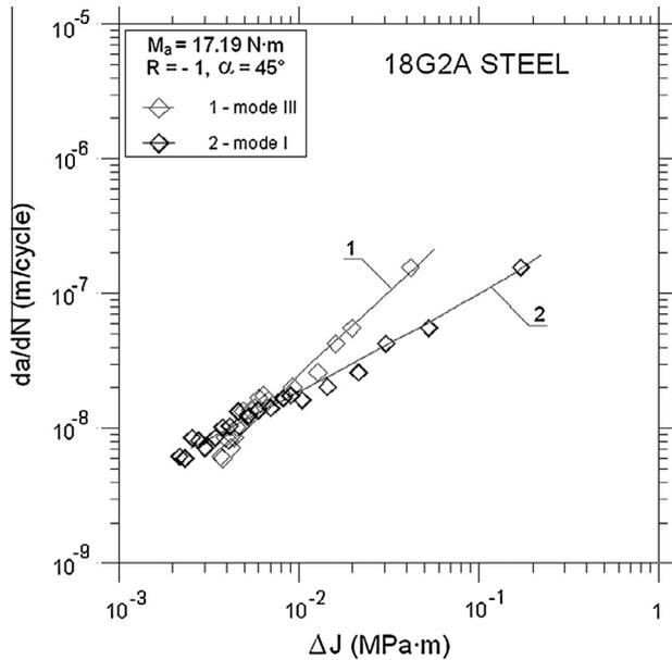
Fig. 12. Fatigue crack growth rate  $da/dN$  versus  $\Delta J$ , for 18G2A steel and  $M_T(t)/M_B(t) = 1$ .
