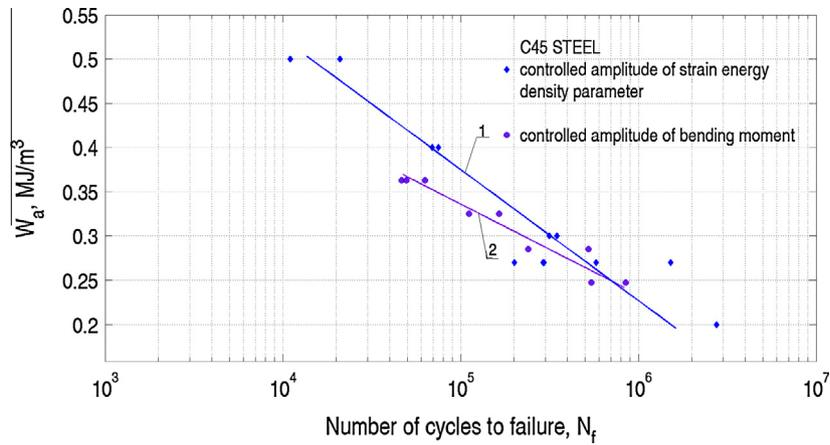
Fig. 9. The fatigue characteristic of C45 steel subjected to bending with a controlled amplitude of the  $\blacklozenge$  – energy parameter with Eq. (26),  $\bullet$  – bending moment (elastic energy).
