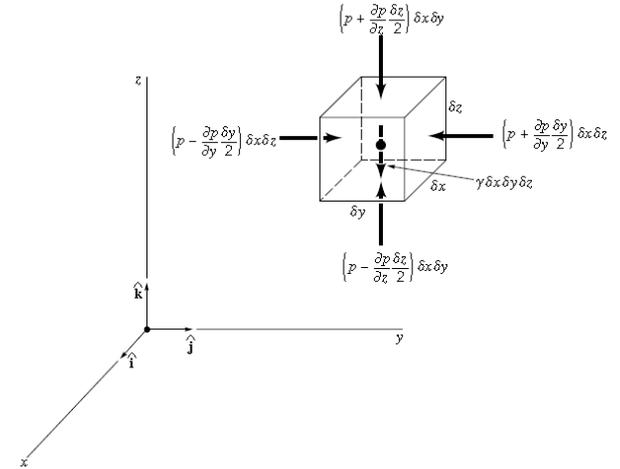
$$\delta F_y = \left( p - \frac{\partial p}{\partial y} \frac{\partial y}{2} \right) \delta x \delta z - \left( p + \frac{\partial p}{\partial y} \frac{\partial y}{2} \right) \delta x \delta z = -\frac{\partial p}{\partial y} \delta x \delta y \delta z \quad (1)$$
