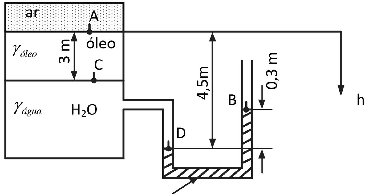
$$p_A = -\gamma_{\text{óleo}} h_C - \gamma_{\text{água}} (h_D - h_C) + \gamma_{\text{Hg}} (h_D - h_B)$$
