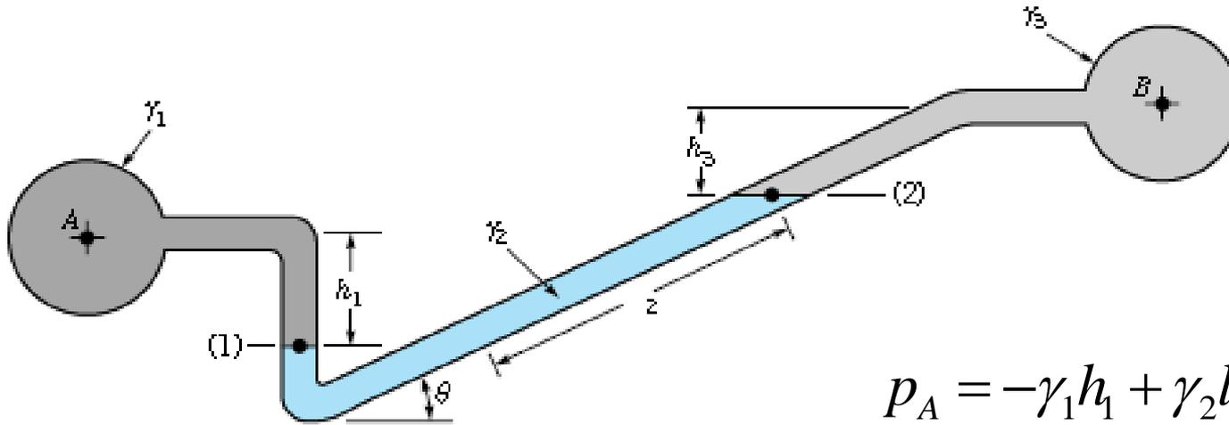
$$p_A = -\gamma_1 h_1 + \gamma_2 l_2 \text{sen}\theta + \gamma_3 h_3 + p_B$$
