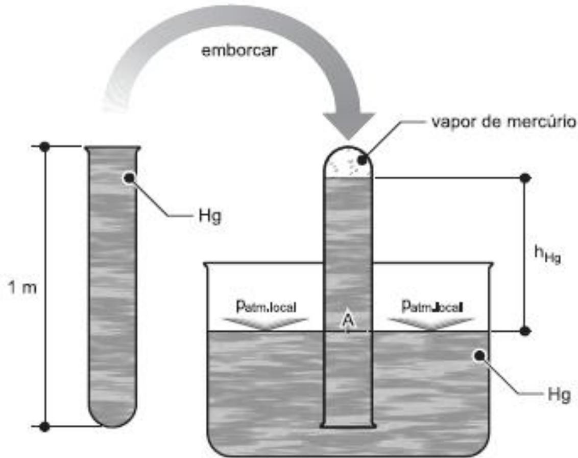
$$p_{atm} = \underbrace{p_{vapor}}_{\text{desprezível}} + \gamma_{Hg} h$$
