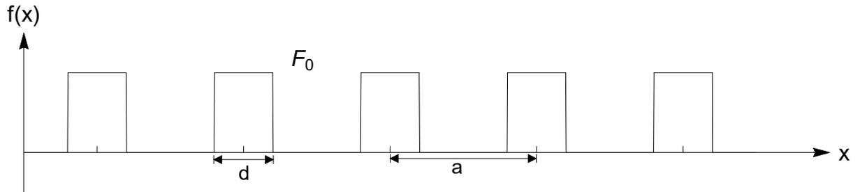
$$a_0 = \frac{1}{a} \int_{-a/2}^{a/2} f(x) dx = \frac{F_0}{a} \int_{-d/2}^{d/2} dx = \frac{d}{a} F_0$$
